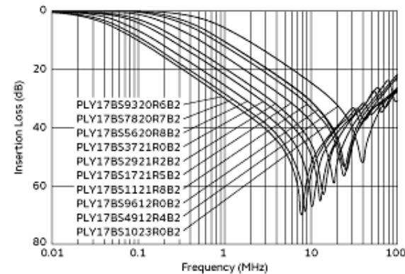
Differential Mode Insertion Loss-Frequency Characteristics
