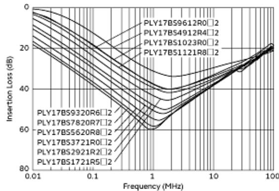
Common Mode Insertion Loss-Frequency Characteristics
