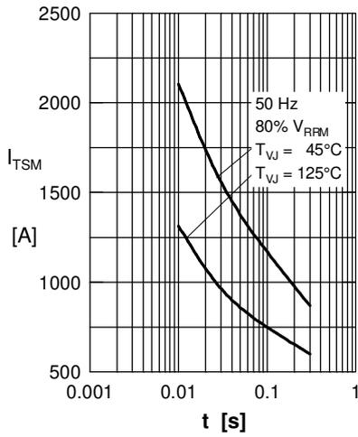
Fig. 1 Surge overload current  $I_{TSM}$ ,
