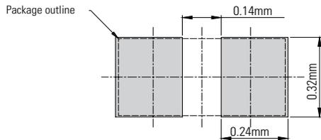
Recommended soldering pad layout
