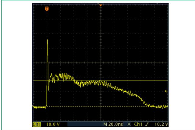
IEC 61000-4-2 -8 kV Contact ESD Clamping Voltage
