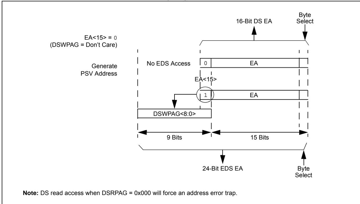
The paged memory scheme provides access to multiple 32-Kbyte windows in the EDS and PSV memory. The Data Space Page registers, DSxPAG, in combination with the upper half of the Data Space address, can provide up to 16 Mbytes of additional address space in the EDS and 8 Mbytes (DSRPAG only) of PSV address space. The paged data memory space is shown in [Figure 4-11](#).
