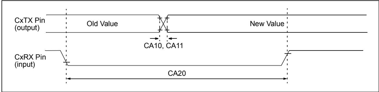
**TABLE 30-48: CANx MODULE I/O TIMING REQUIREMENTS**
