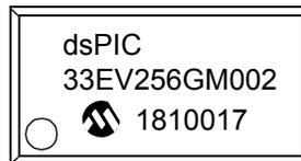
28-Lead QFN-S (6x6x0.9 mm)
