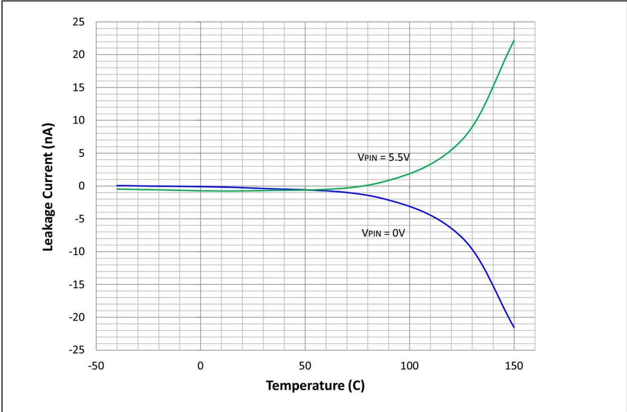
FIGURE 32-26: TYPICAL I<sub>IL</sub> vs. TEMPERATURE (GENERAL PURPOSE I/Os)
