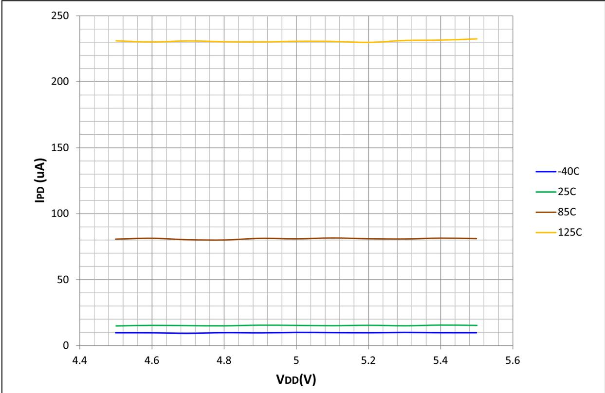
FIGURE 32-18: TYPICAL/MAXIMUM IPD vs. TEMPERATURE
