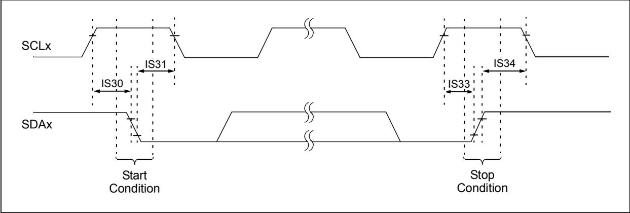
**FIGURE 30-31: I2Cx BUS DATA TIMING CHARACTERISTICS (SLAVE MODE)**
