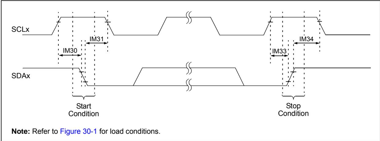
**FIGURE 30-29: I2Cx BUS DATA TIMING CHARACTERISTICS (MASTER MODE)**
