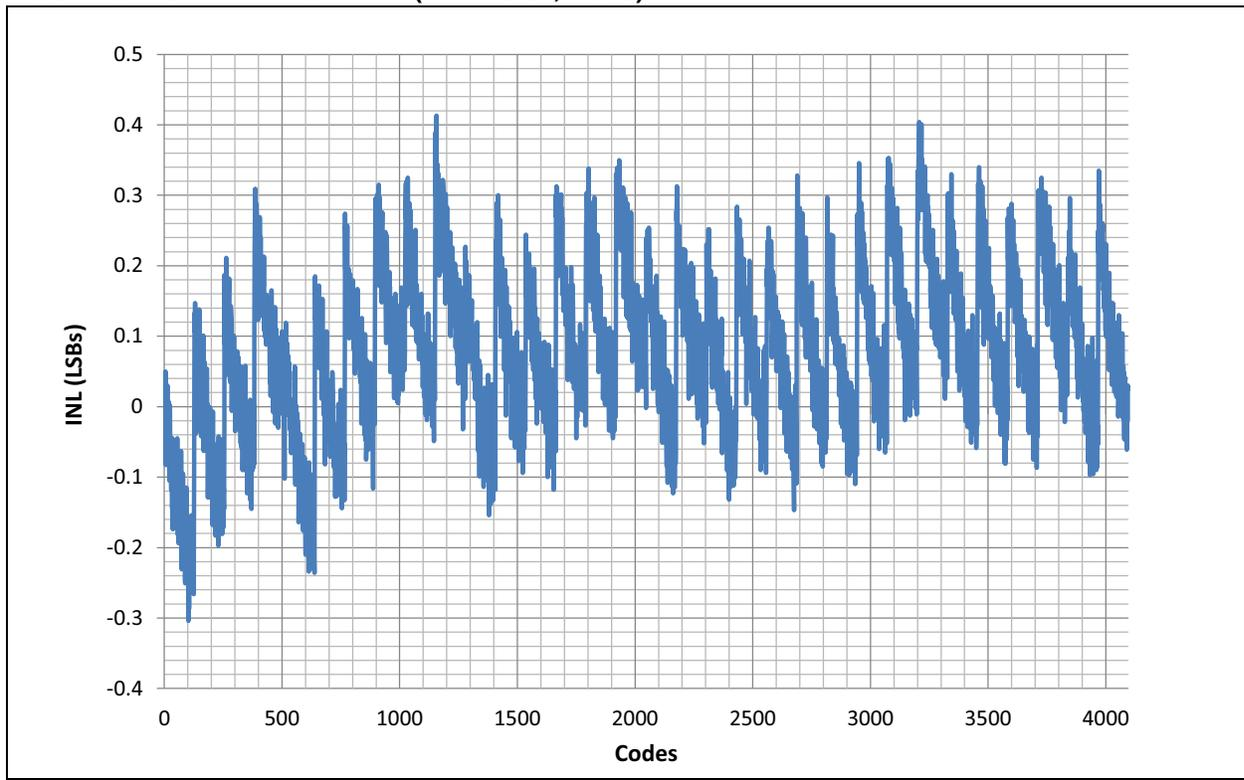
FIGURE 32-46: TYPICAL INL ( $V_{DD} = 5.5V, +25^{\circ}C$ )
