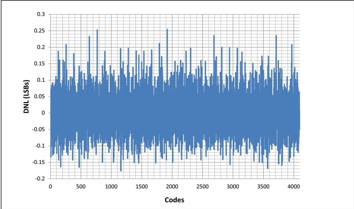
FIGURE 32-42: TYPICAL DNL ( $V_{DD} = 5.5V, +25^{\circ}C$ )
