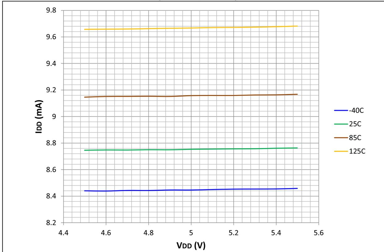
FIGURE 32-4: TYPICAL  $I_{DD}$  vs.  $V_{DD}$  (EC MODE, 40 MIPS)
