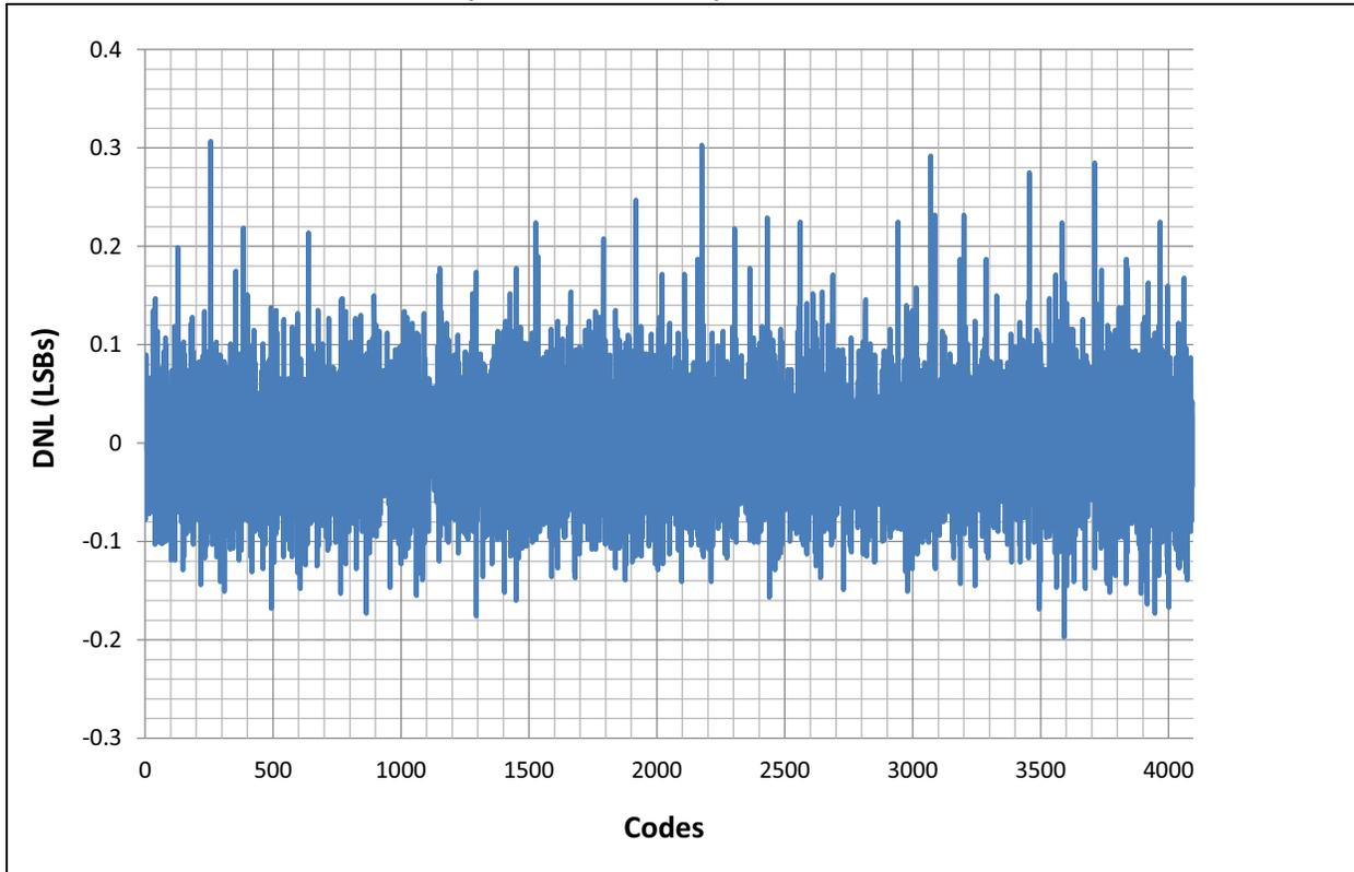
FIGURE 32-44: TYPICAL DNL ( $V_{DD} = 5.5V, +125^{\circ}C$ )
