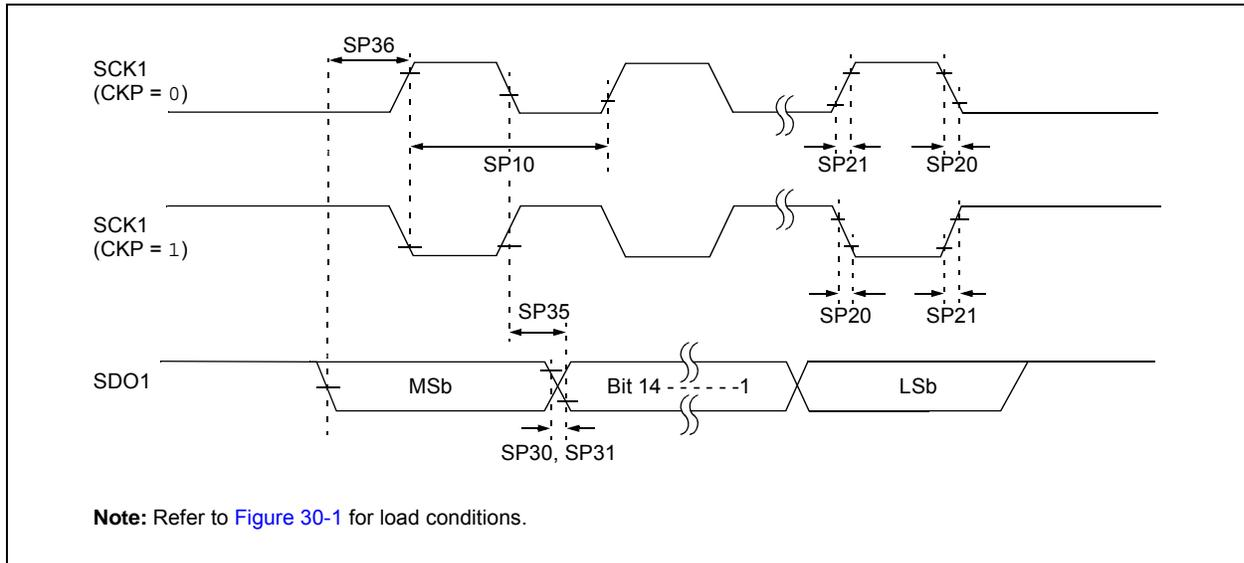
**TABLE 30-39: SPI1 MASTER MODE (HALF-DUPLEX, TRANSMIT ONLY) TIMING REQUIREMENTS**
