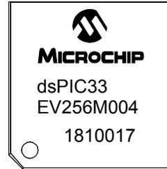
44-Lead QFN (8x8 mm)
