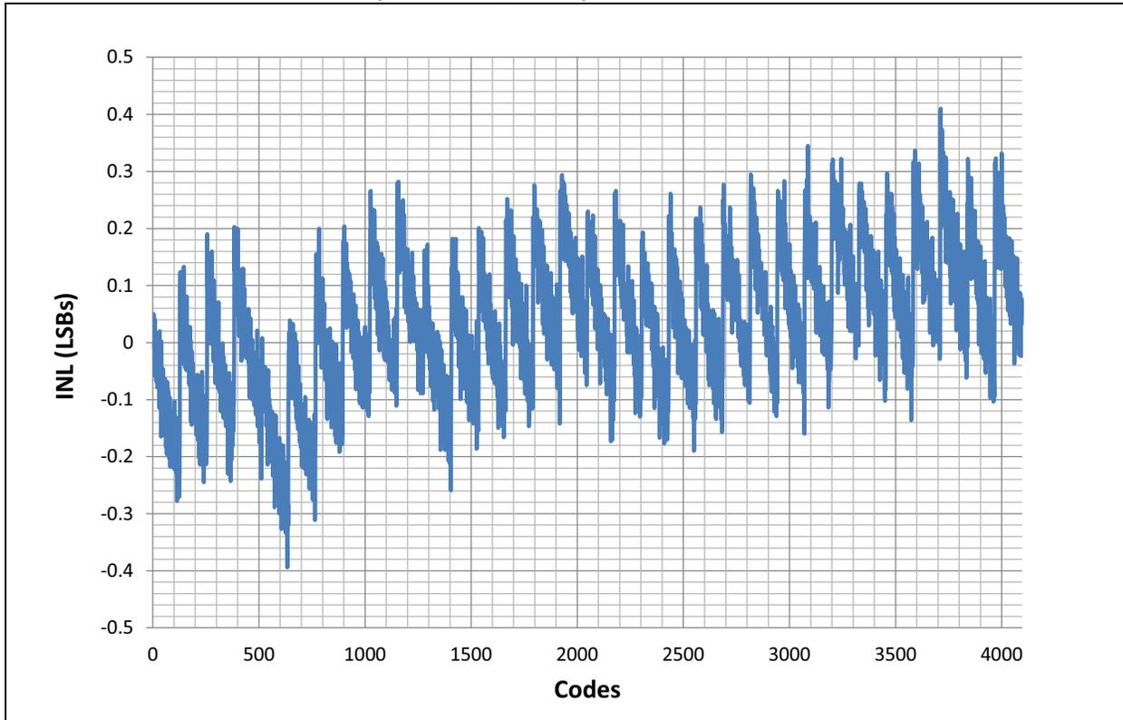
FIGURE 32-48: TYPICAL INL ( $V_{DD} = 5.5V, +125^{\circ}C$ )
