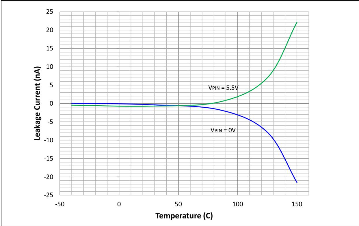
FIGURE 33-22: TYPICAL I<sub>IL</sub> vs. TEMPERATURE (GENERAL PURPOSE I/Os)
