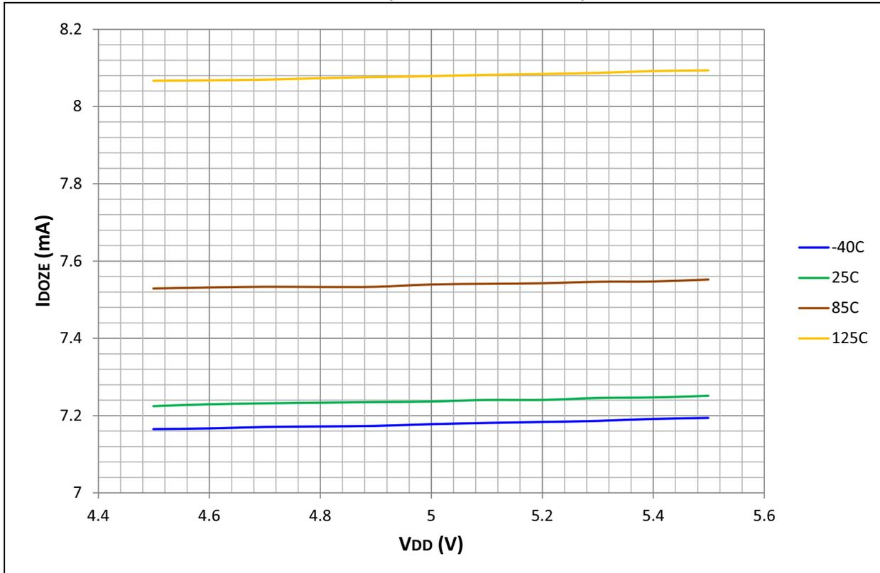
FIGURE 32-16: TYPICAL/MAXIMUM I<sub>DOZE</sub> vs. TEMPERATURE (DOZE 1:128, 70 MIPS)
