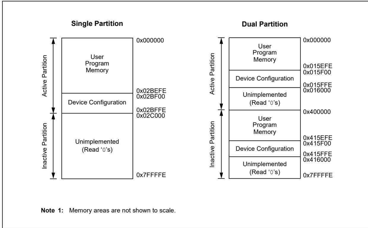
**FIGURE 4-3: PROGRAM MEMORY MAP FOR dsPIC33CK128MP50X/20X DEVICES<sup>(1)</sup>**
