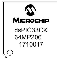
64-Lead QFN (9x9x0.9 mm)
