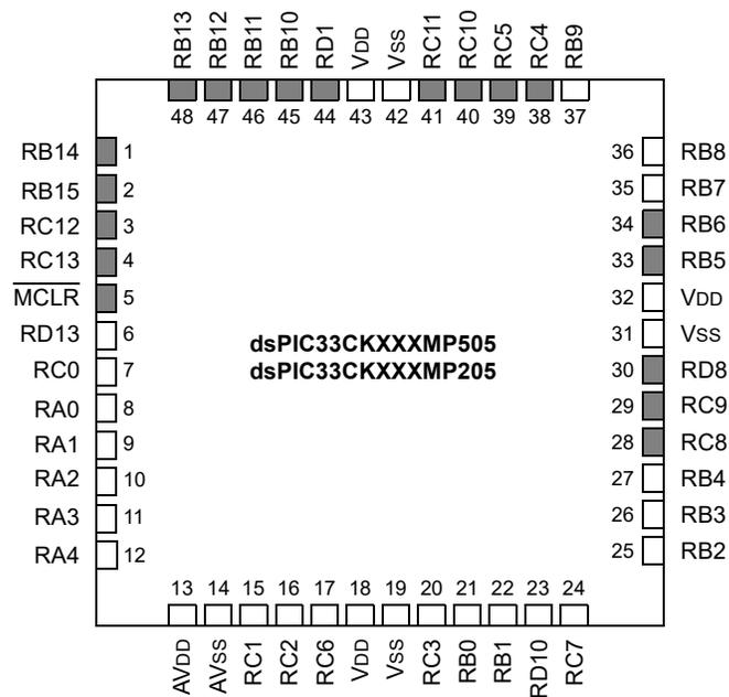
**Note 1:** Shaded pins are up to 5 VDC tolerant.
