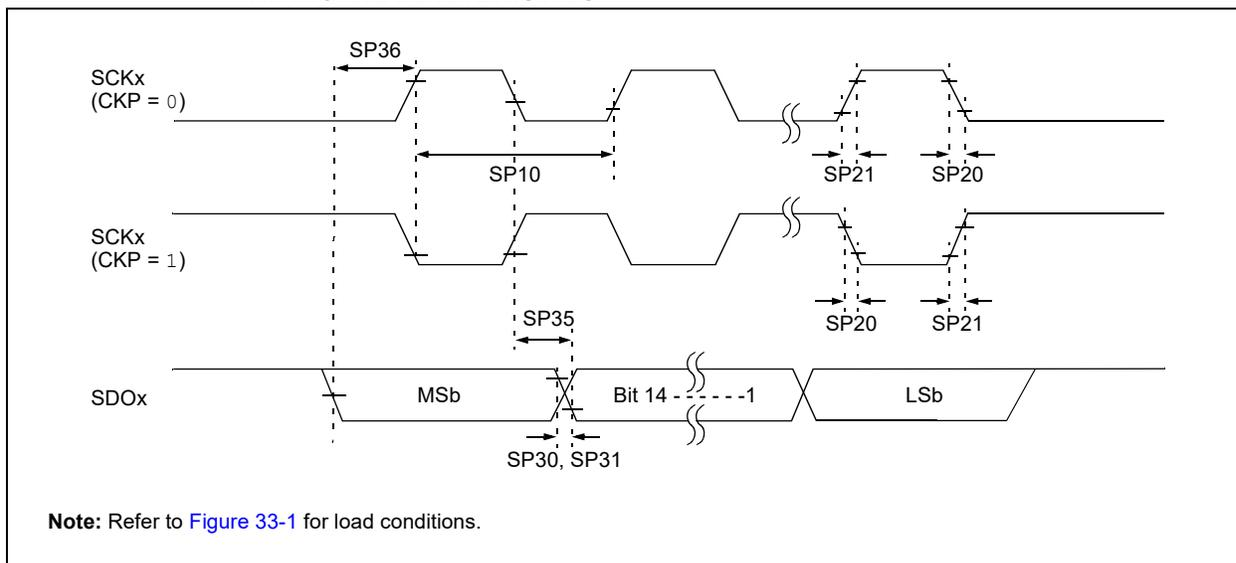
**TABLE 33-28: SPIx MASTER MODE (HALF-DUPLEX, TRANSMIT ONLY) TIMING REQUIREMENTS**
