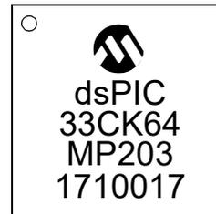
48-Lead TQFP (7x7 mm)
