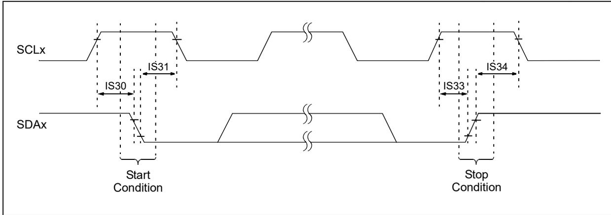
**FIGURE 33-16: I2Cx BUS DATA TIMING CHARACTERISTICS (SLAVE MODE)**
