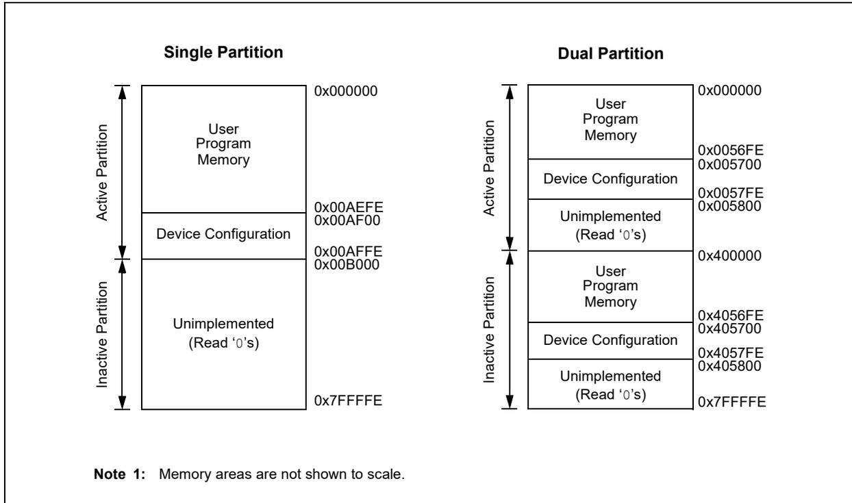
**FIGURE 4-5: PROGRAM MEMORY MAP FOR dsPIC33CK32MP50X/20X DEVICES<sup>(1)</sup>**
