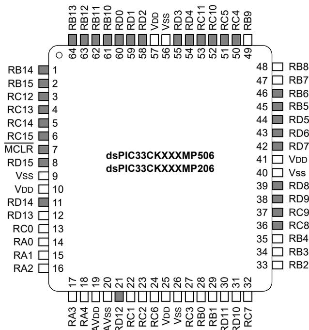
**Note:** Shaded pins are up to 5 VDC tolerant.
