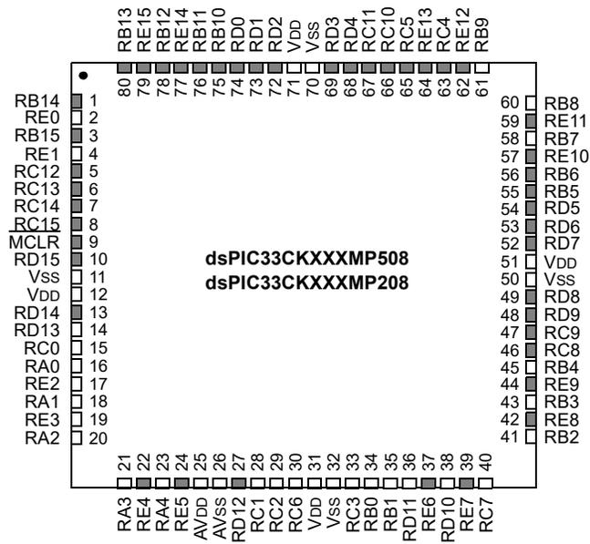
**Note:** Shaded pins are up to 5 VDC tolerant.
