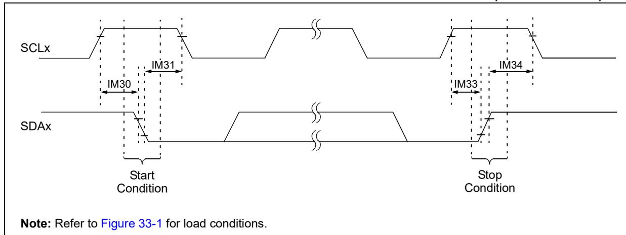
**FIGURE 33-14: I2Cx BUS DATA TIMING CHARACTERISTICS (MASTER MODE)**
