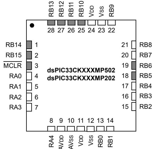
**Note 1:** Shaded pins are up to 5 VDC tolerant.
