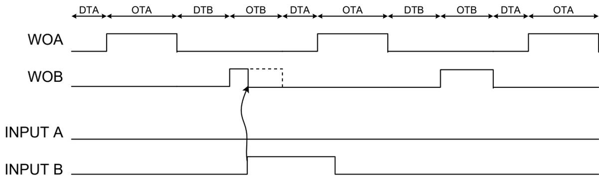
**Input Mode 10: Stop Output on Edge, Maintain Frequency**
