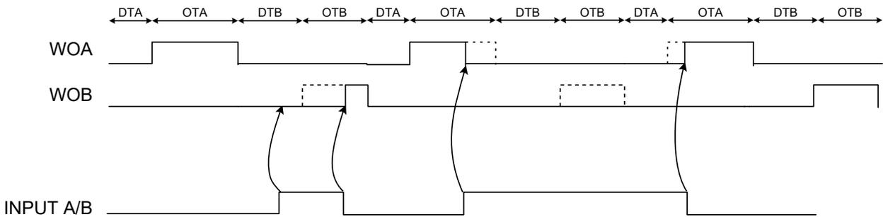
**Input Mode 5: Stop all Outputs, Execute Dead Time while Fault Active**
