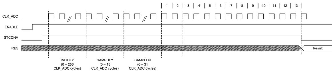
In Free Running mode, a new conversion will be started immediately after the conversion completes, while the STCONV bit is one. The sampling rate  $R_S$  in free running mode is calculated by
