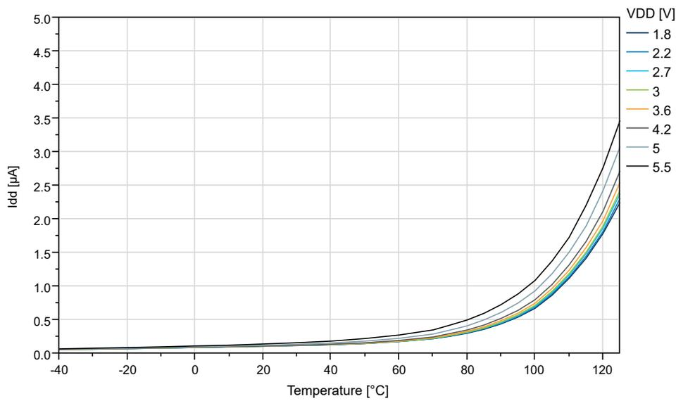
**Figure 35-11. Power Down Mode Supply Current vs.  $V_{DD}$  (all functions disabled)**
