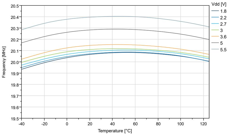
Figure 35-59. OSC20M Internal Oscillator: Frequency vs.  $V_{DD}$
