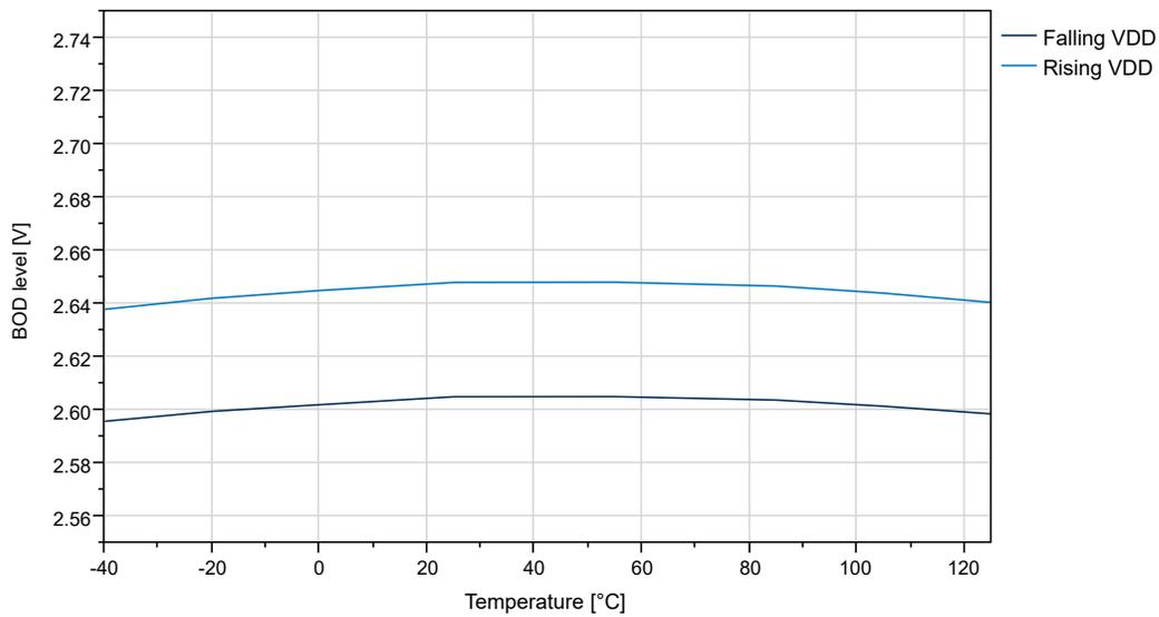
Figure 35-41. BOD Threshold vs. Temperature (Level 4.3V)
