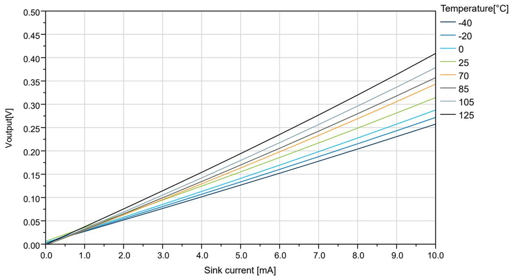
Figure 35-23. IO Pin Output Voltage vs. Sink Current ( $V_{DD}=5.0V$ )
