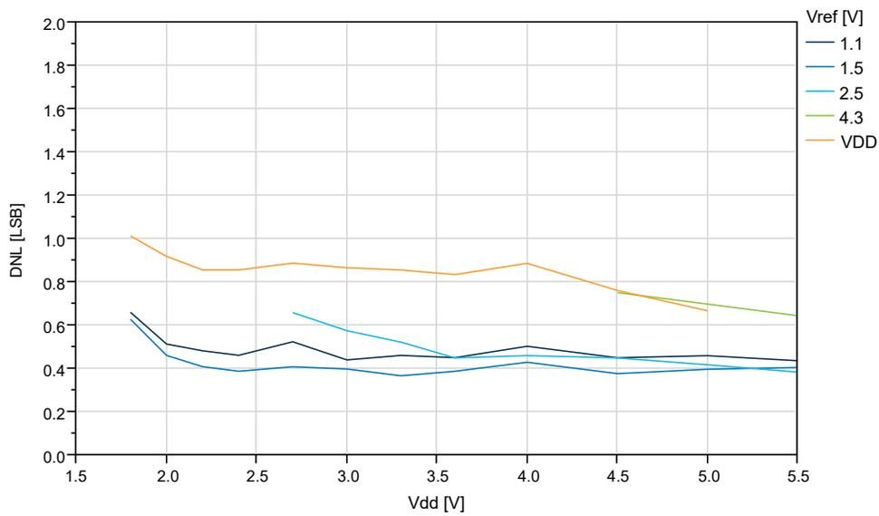
**Figure 35-45. DNL vs.  $V_{ref}$  ( $V_{DD}=5.0V$ , 115ksp/s)**
