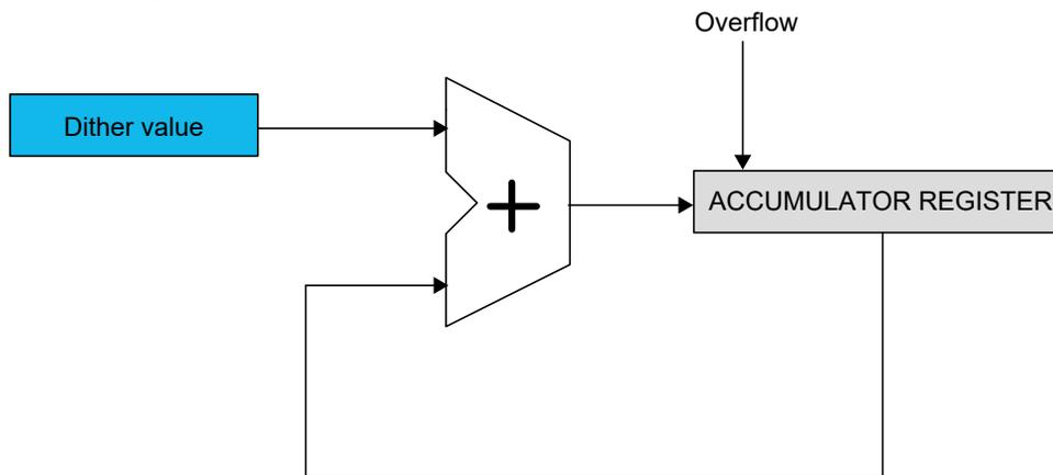
The user can select where in the TCD cycle the dither will be added by writing to the Dither Selection bits in the Dither Control register (DITHERSEL in TCD.DITCTRL):
