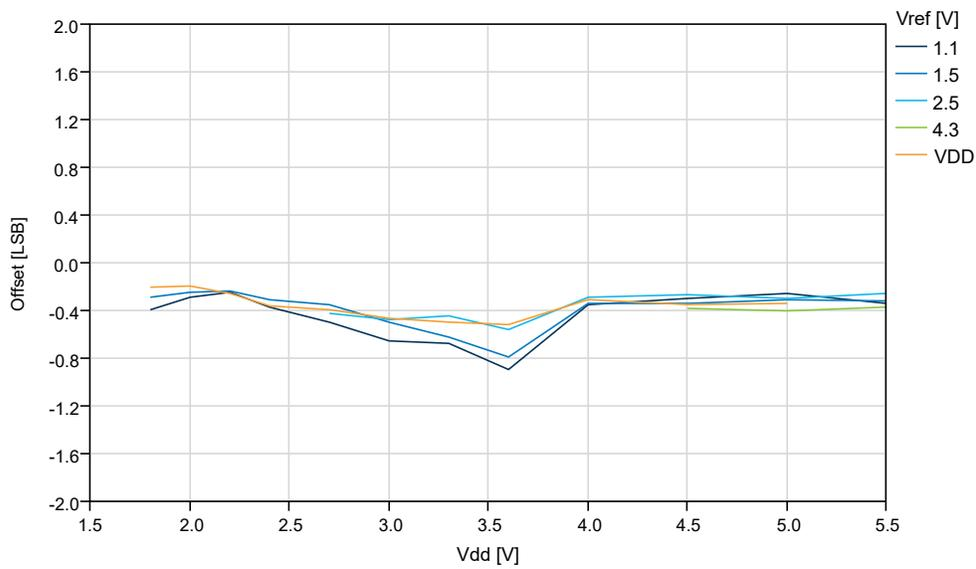
Figure 35-51. Offset Error vs.  $V_{ref}$  ( $V_{DD}=5.0V$ , 115ksps)
