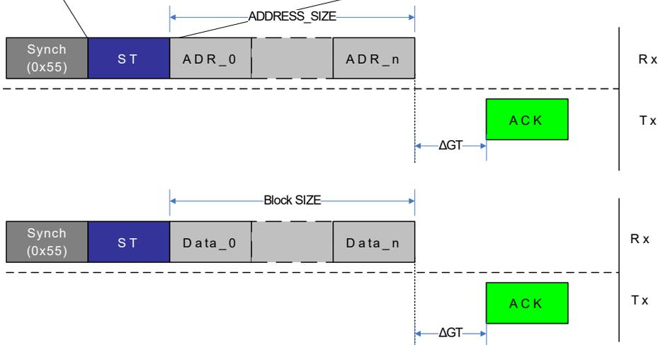
The Figure above gives an example of `ST` to the UPDI pointer register, and store of regular data. In both cases an Acknowledge (ACK) is sent back by the UPDI if the store was successful, and a SYNCH character is sent before each instruction. To write the UPDI pointer register, the following procedure should be followed.
