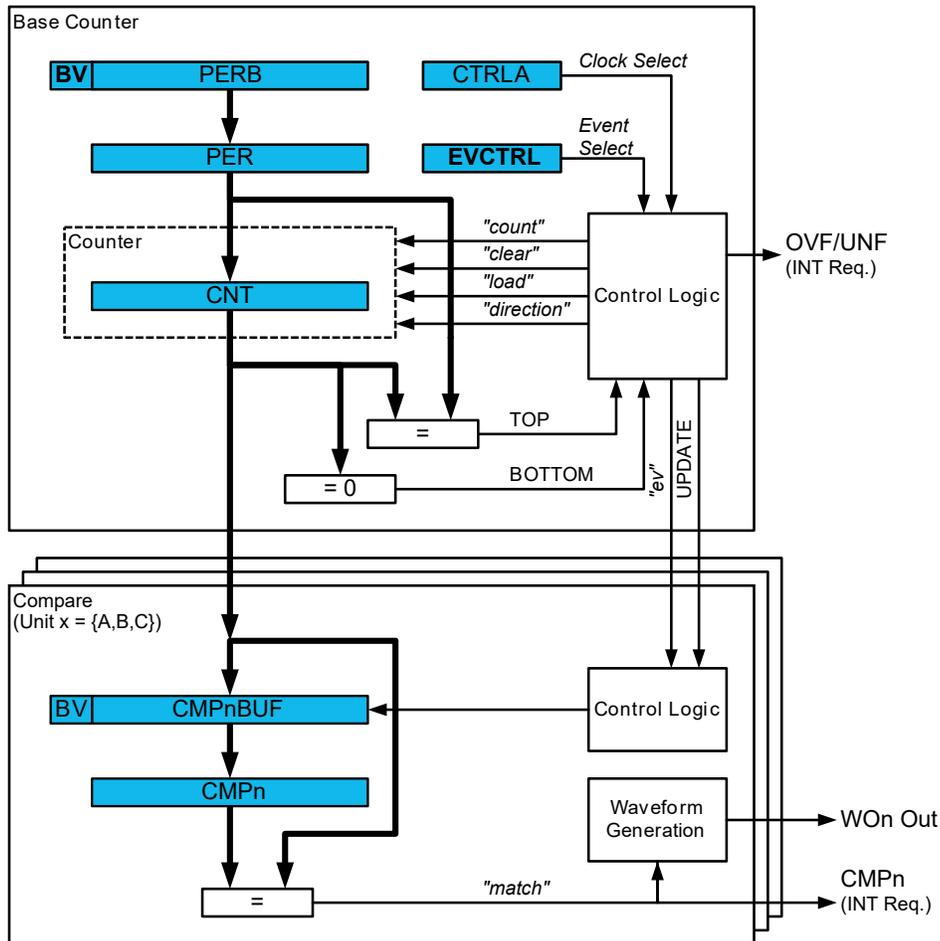
The counter register (CNT), period registers with buffer (PER and PERBUF), and compare registers with buffers (CMPx and CMPBUFx) are 16-bit registers. All buffer registers have a buffer valid (BV) flag that indicates when the buffer contains a new value.
