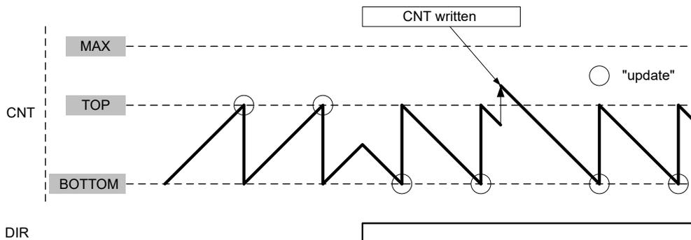
It is possible to change the Counter value in the Counter register (TCA.CNT) when the counter is running. The write access to TCA.CNT has higher priority than count, clear, or reload, and will be immediate. The direction of the counter can also be changed during normal operation by writing to DIR in TCA.CTRLE.
