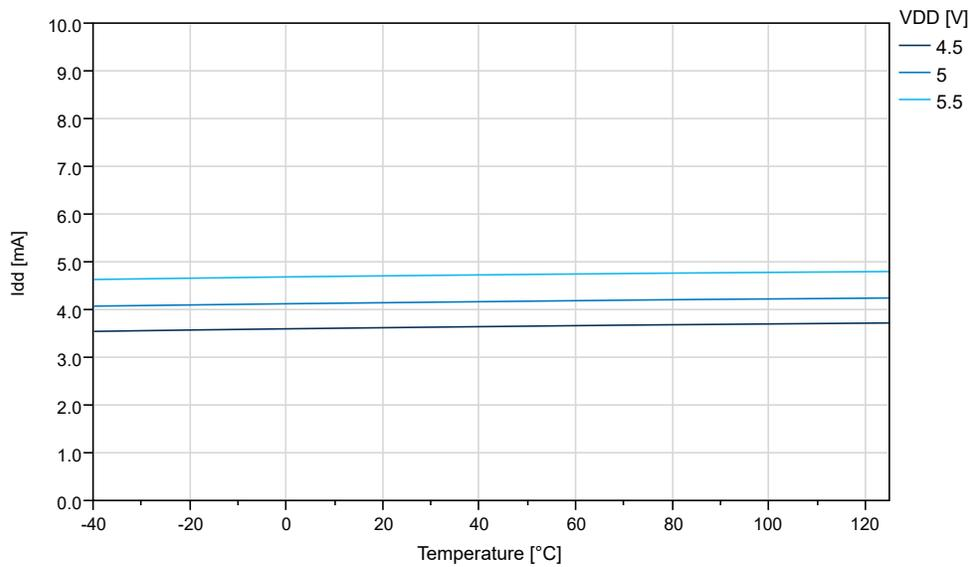
**Figure 35-9. Idle Supply Current vs.  $V_{DD}$  ( $f=32\text{KHz OSCULP32K}$ )**
