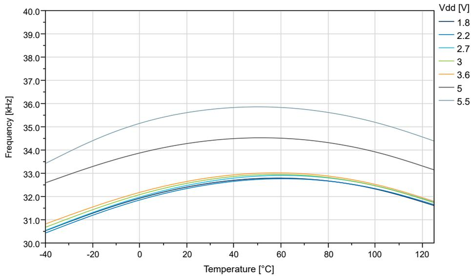
Figure 35-61. OSCULP32K Internal Oscillator Frequency vs.  $V_{DD}$
