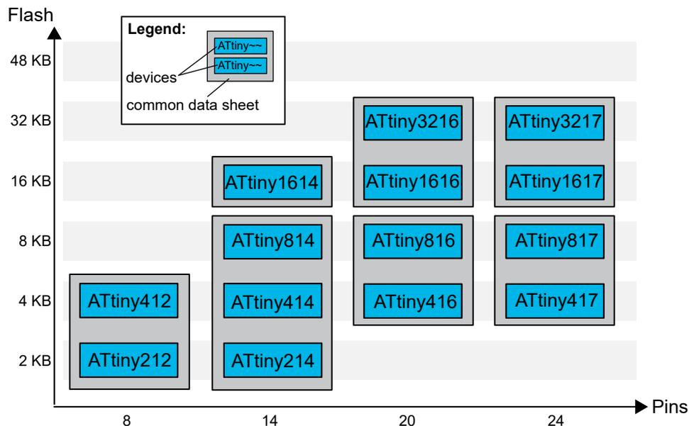
Devices with different Flash memory size typically also have different SRAM and EEPROM.
