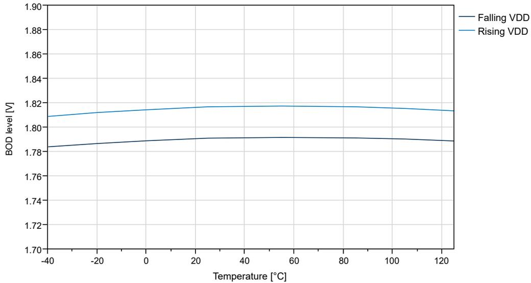
Figure 35-40. BOD Threshold vs. Temperature (Level 2.6V)
