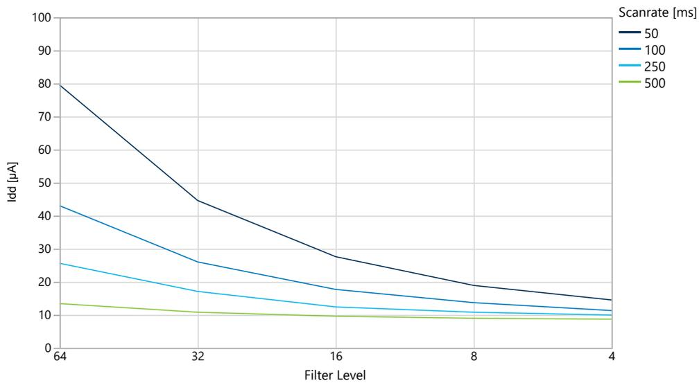
Figure 35-64.  $I_{DD}$  vs Temperature over Scanrates. Filterlevel = 16,  $V_{DD} = 3.0\text{V}$ , Drift cal off.
