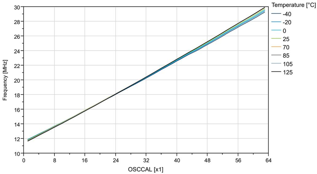
**Figure 35-58. OSC20M Internal Oscillator: Frequency vs. Temperature**
