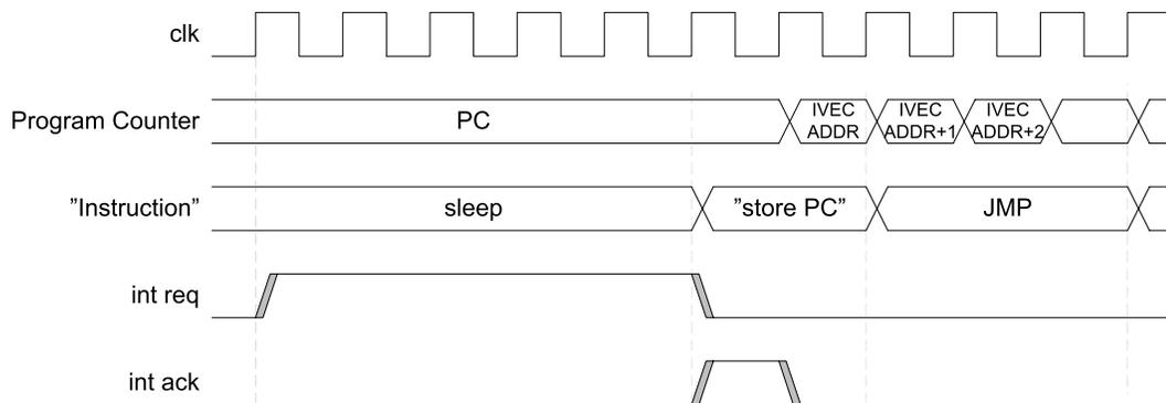
If an interrupt occurs when the device is in sleep mode, the interrupt execution response time is increased by five clock cycles. In addition, the response time is increased by the start-up time from the selected sleep mode.
