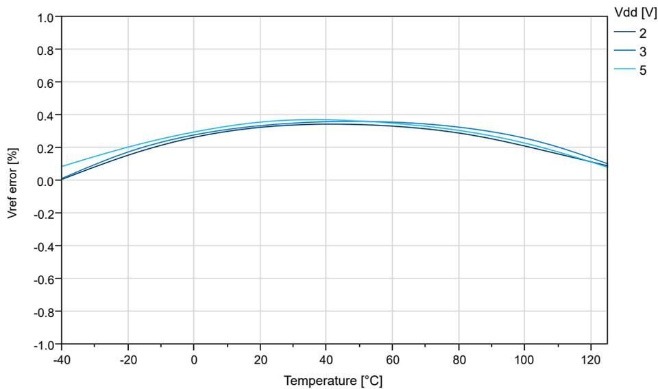
Figure 35-33. Internal 1.1V Reference vs. Temperature
