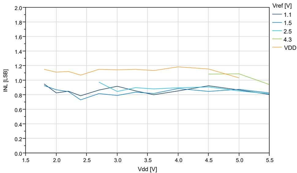
**Figure 35-49. INL vs.  $V_{ref}$  ( $V_{DD}=5.0V$ , 115ksps)**
