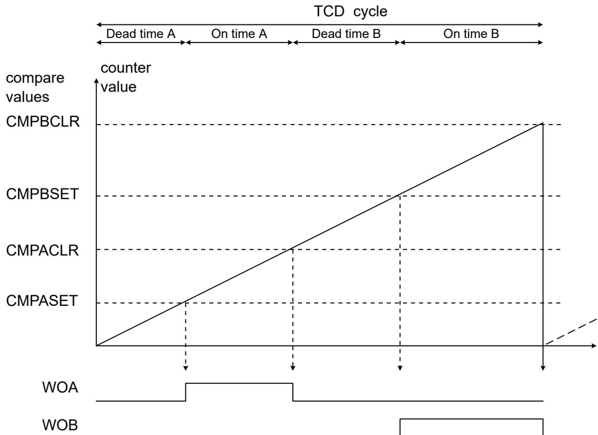
In the figure above,  $\text{CMPASET} < \text{CMPACLR} < \text{CMPBSET} < \text{CMPBCLR}$ . This is required in One Ramp Mode to avoid overlapping outputs. The figure below is an example where  $\text{CMPBSET} < \text{CMPASET} < \text{CMPACLR} < \text{CMPBCLR}$ , resulting in an overlap of the outputs.
