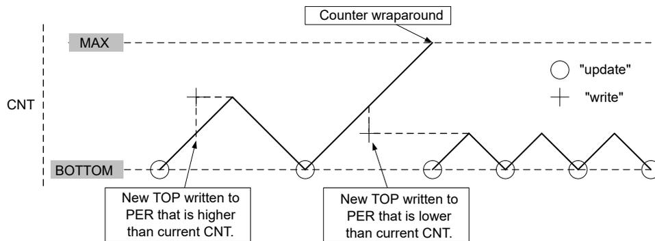
**With Buffering:** When double buffering is used, the buffer can be written at any time and still maintain correct operation. The TCA.PER is always updated on the UPDATE condition, as shown for dual-slope operation in the figure below. This prevents wraparound and the generation of odd waveforms.
