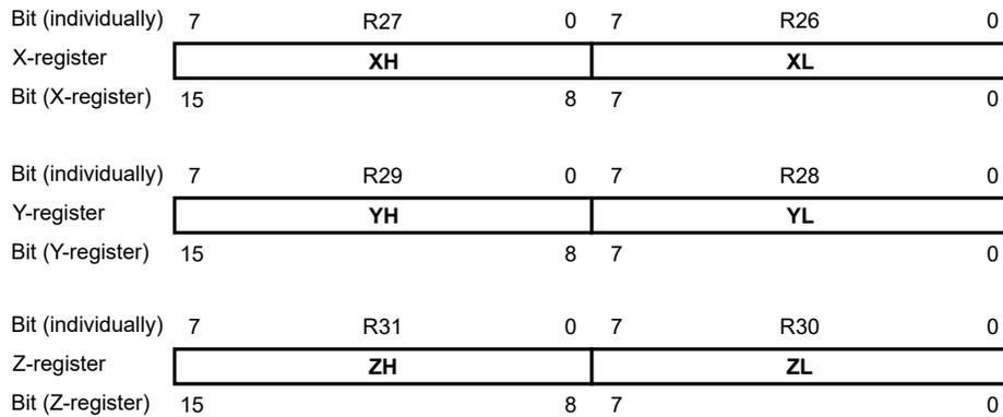
The lowest register address holds the least-significant byte (LSB), and the highest register address holds the most-significant byte (MSB). In the different addressing modes, these address registers function as fixed displacement, automatic increment, and automatic decrement.
