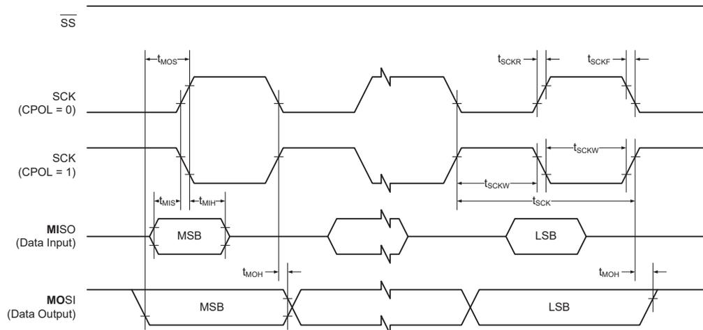
**Figure 34-6. SPI - Timing Requirements in Slave Mode**
