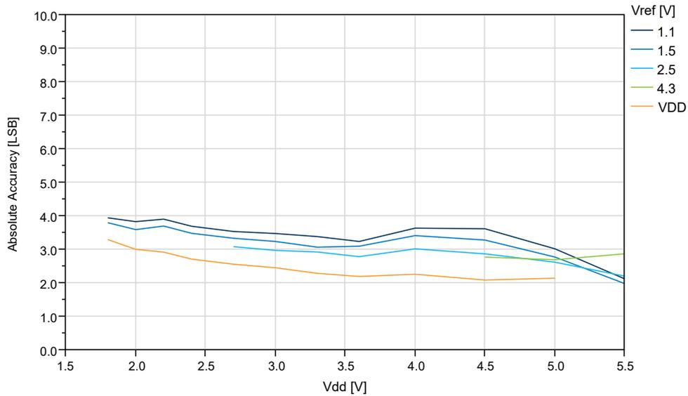
**Figure 35-43. Absolute Accuracy vs.  $V_{ref}$  ( $V_{DD}=5.0V$ , 115kps)**
