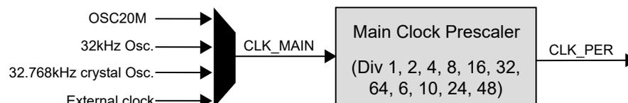
The Main Clock and Prescaler configuration registers (CLKCTRL.MCLKCTRLA, CLKCTRL.MCLKCTRLB) are protected by the Configuration Change Protection Mechanism, employing a timed write procedure for changing these registers.
