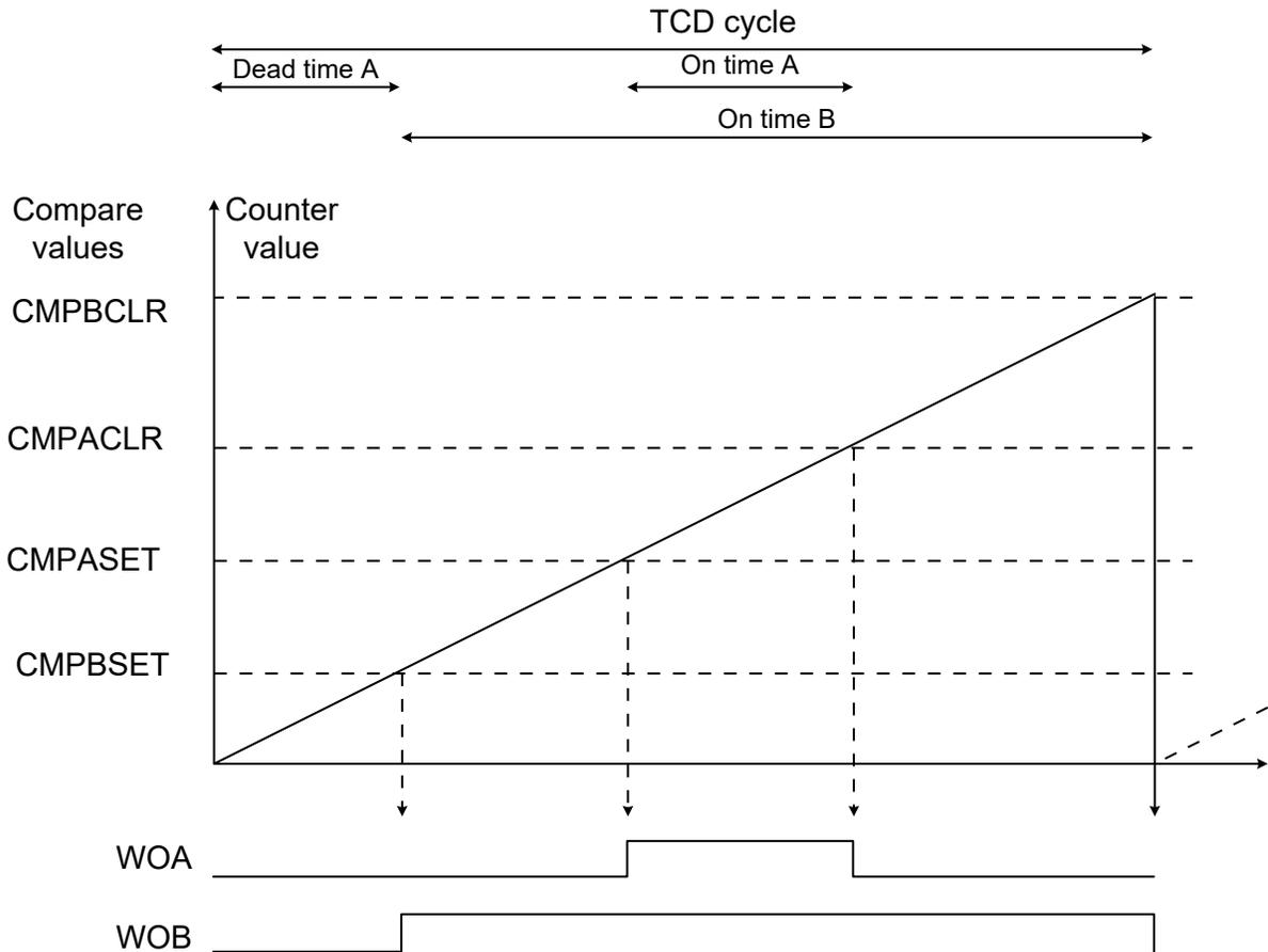
If any of the other compare values are bigger than CMPBCLR it will never be triggered when running in One ramp mode. And if The CMPACL is smaller than the CMPASET value, the clear value will not have any effect.
