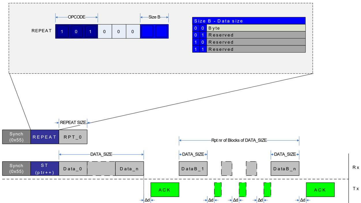
The Figure above gives an example of repeat operation with a ST instruction using pointer post increment operation. After the REPEAT instruction is sent with RPT\_0 = n, the first ST instruction is issued with SYNCH- and Instruction frame, while the next n ST-instructions are executed by only sending in data bytes according to the ST operand DATA\_SIZE, and maintaining the Acknowledge (ACK) handshake protocol.
