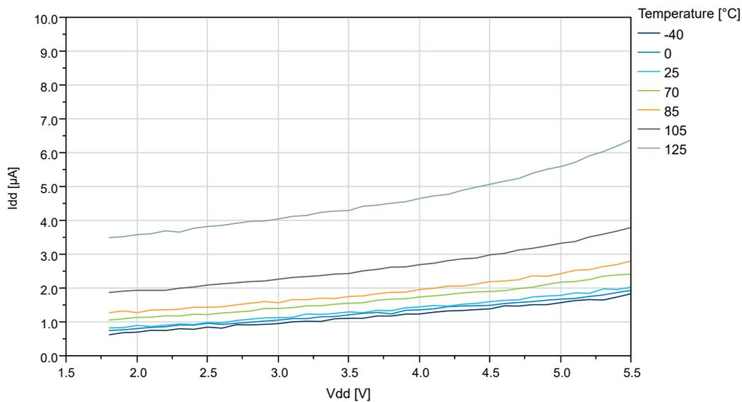
**Figure 35-13. Standby Mode Supply Current vs.  $V_{DD}$  (RTC running with internal OSCULP32K)**
