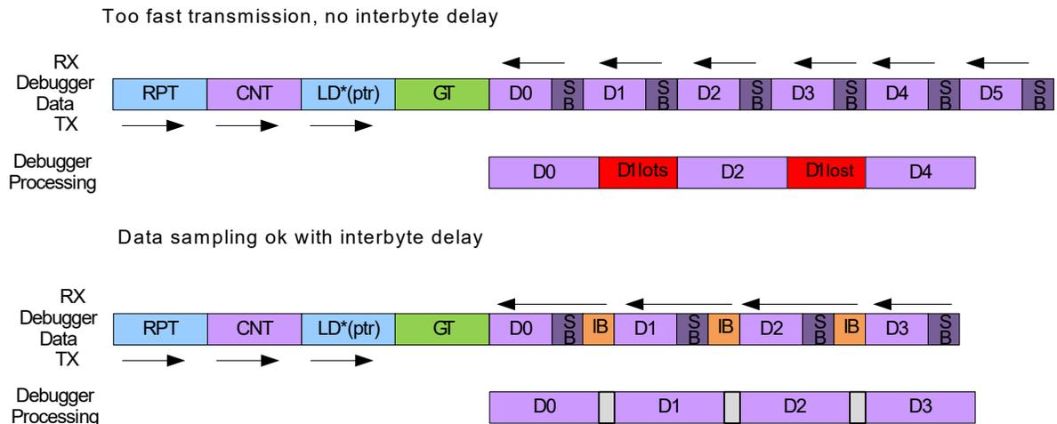
In [Figure 33-18](#), GT denotes the Guard Time insertion, SB are stop bits and IB is the inserted interbyte delay. The rest of the frames are data and instructions.
