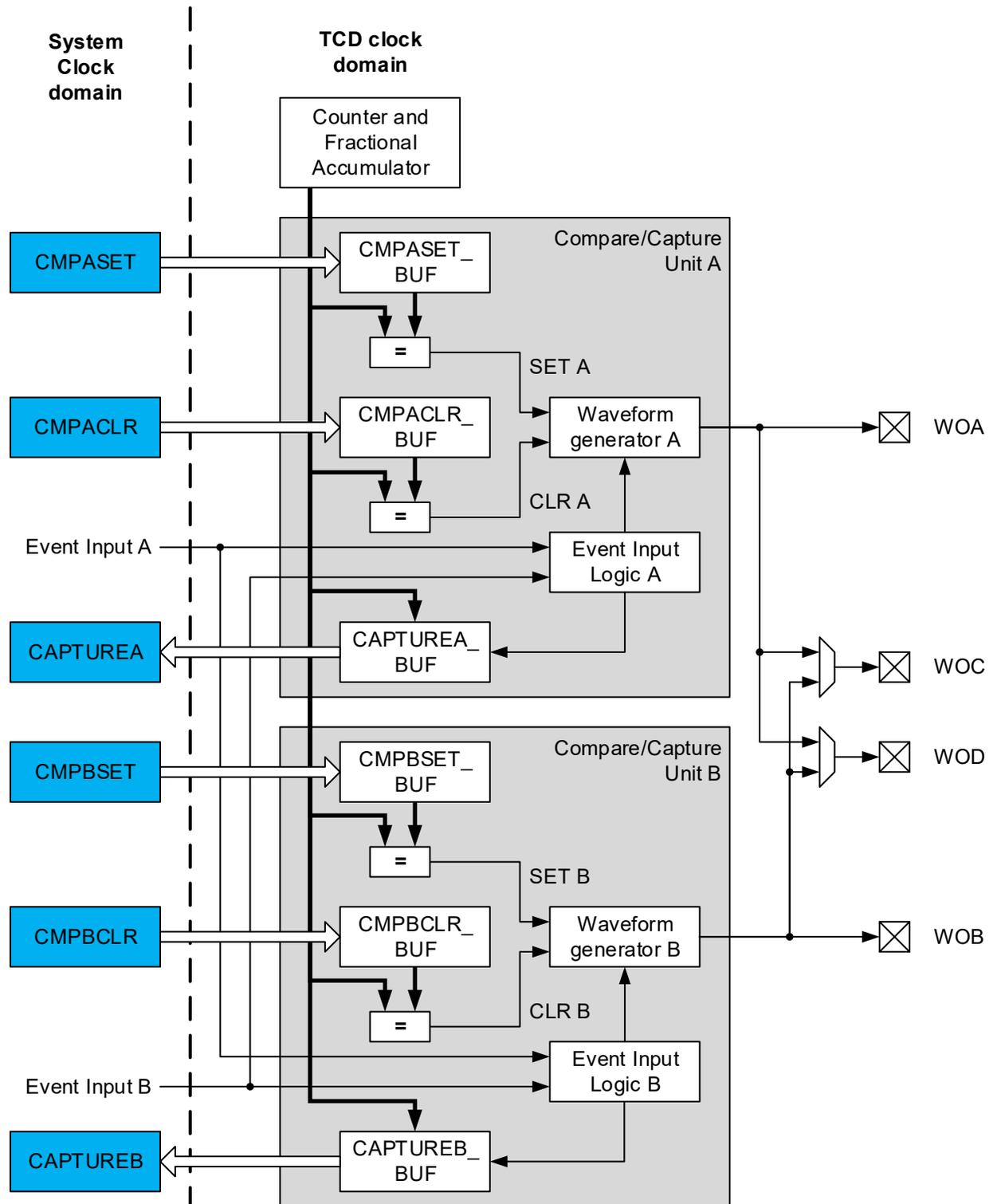
The TCD core is asynchronous to the system clock. The timer/counter consist of two compare/capture units, each with a separate waveform output. In addition there are two extra waveform outputs which can be equal to the output from one of the units. The compare registers CMPxSET, CMPxCLR are stored in the respective registers
