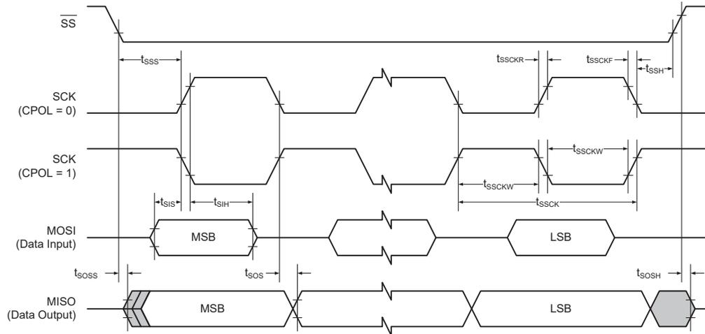
**Table 34-17. USART in SPI Mode - Timing Characteristics**
