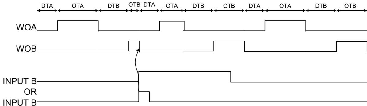
**Input Mode 9: Stop Output at Level, Maintain Frequency**
