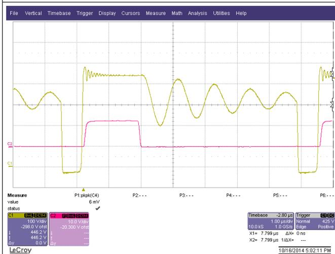
C2(RED): DRV signal to synchronous rectifier Q1
