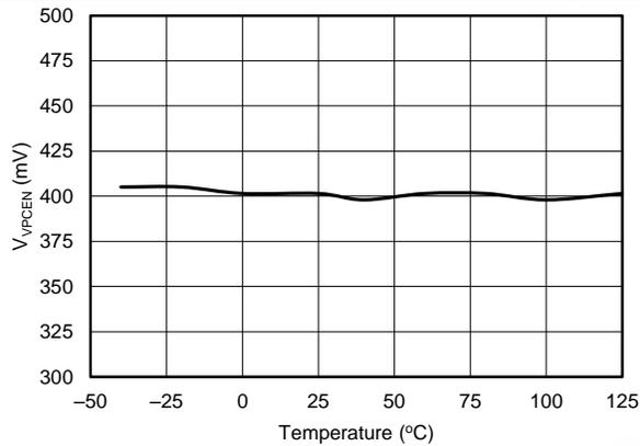
Figure 3. VPC Enable Threshold vs Temperature
