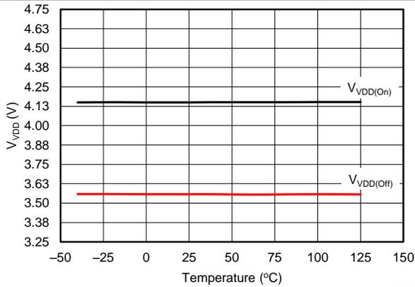
Figure 1. VDD Turn-On and Turn-Off Threshold vs Temperature
