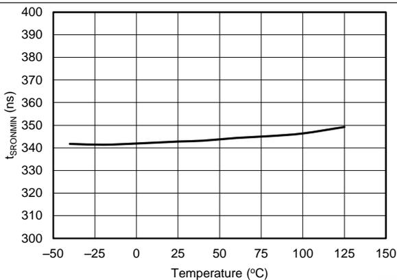
**Figure 11. DRV Minimum On Time vs Temperature**
