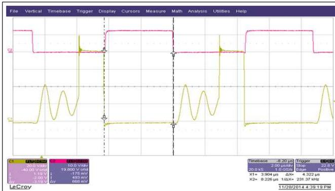
C2(RED): DRV signal to synchronous rectifier Q1
