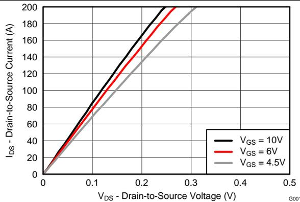
Figure 2. Saturation Characteristics
