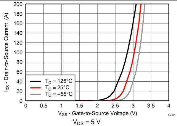
Figure 3. Transfer Characteristics
