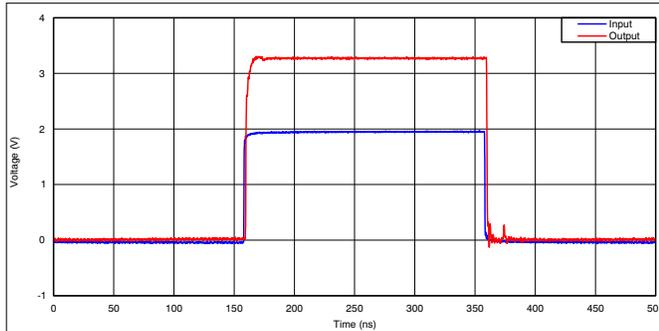
图 9-4. Captured Waveform From Above I<sup>2</sup>C Set-Up (1.8 V to 3.3 V at 2.5 MHz)
