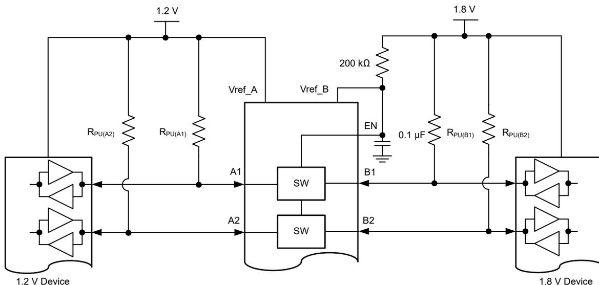
图 9-8. 1.2 V to 1.8 V Level Translation with LSF0108-Q1
