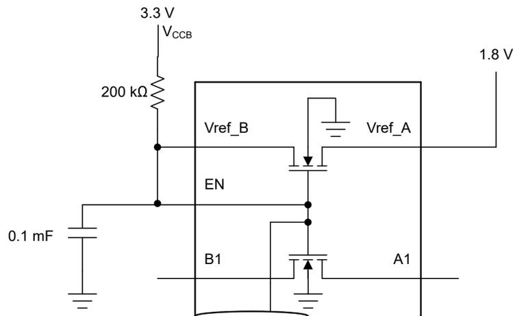
**图 9-2. Bias Circuitry Inside the LSF0108-Q1 Devices**
