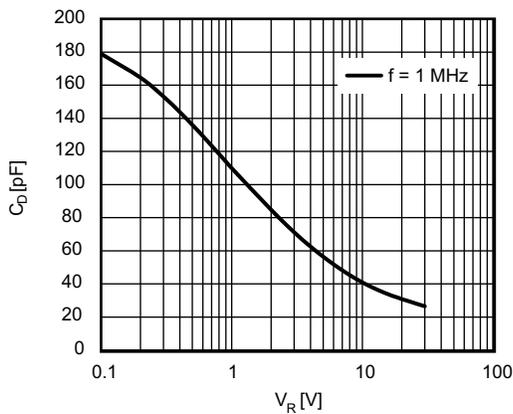
Fig. 2 - Typical Diode Capacitance vs. Reverse Voltage
