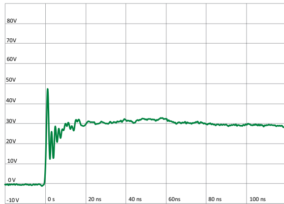
IEC 61000-4-2 +8 kV Contact ESD Clamping Voltage
