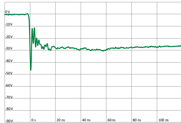
IEC 61000-4-2 -8 kV Contact ESD Clamping Voltage
