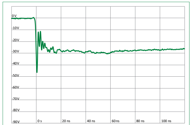
IEC 61000-4-2 -8 kV Contact ESD Clamping Voltage
