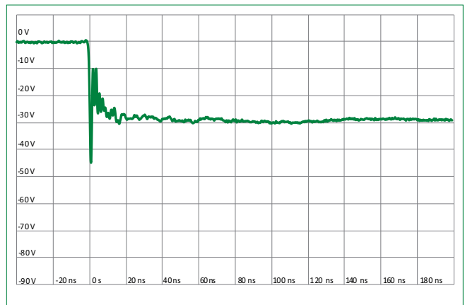
ISO10605 Contact Discharge Plot at -8 kV
