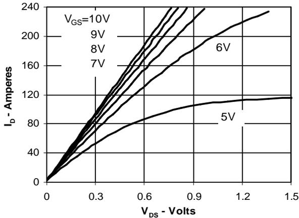
**Fig. 2. Output Characteristics @ 125 Deg. C**
