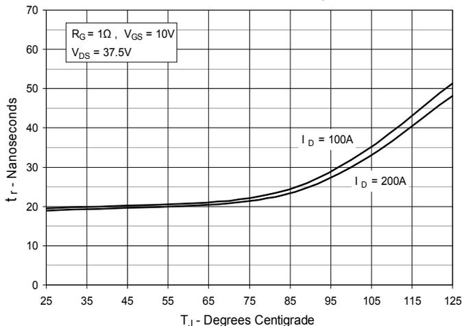
**Fig. 14. Resistive Turn-on Rise Time vs. Drain Current**
