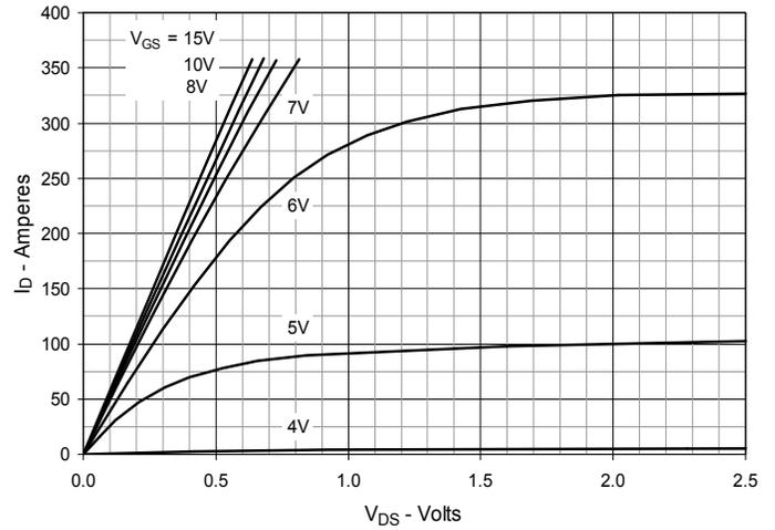
Fig. 3. Output Characteristics @  $T_J = 150^\circ\text{C}$
