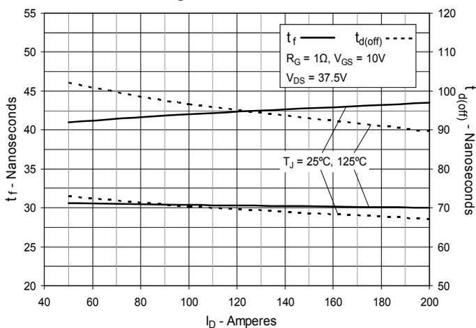
**Fig. 18. Resistive Turn-off Switching Times vs. Gate Resistance**
