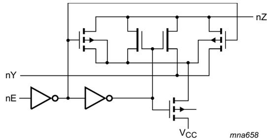
Fig 3. Logic diagram (one switch)
