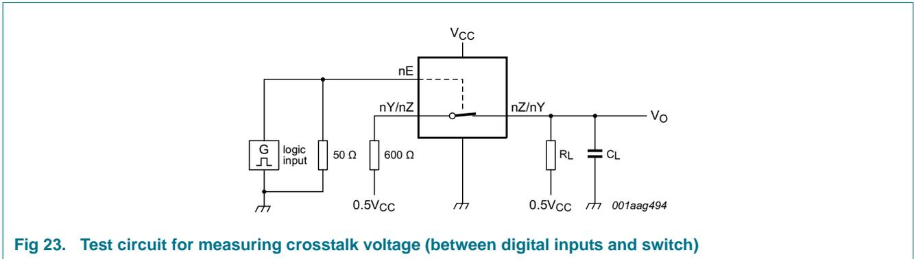
Fig 23. Test circuit for measuring crosstalk voltage (between digital inputs and switch)
