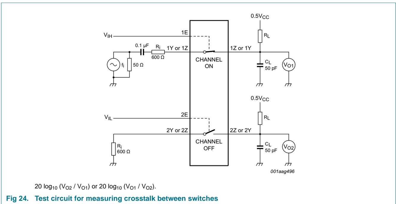
$20 \log_{10} (V_{O2} / V_{O1})$  or  $20 \log_{10} (V_{O1} / V_{O2})$ .
