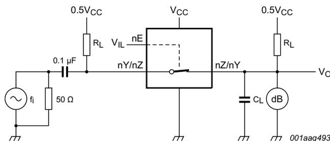
Adjust  $f_i$  voltage to obtain 0 dBm level at input.
