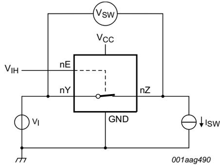
$R_{ON} = V_{SW} / I_{SW}$ .
