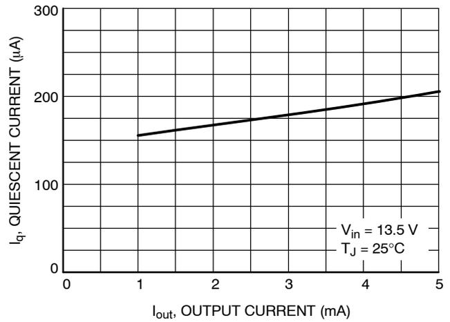
Figure 9. Quiescent Current vs. Output Current (Low Load)
