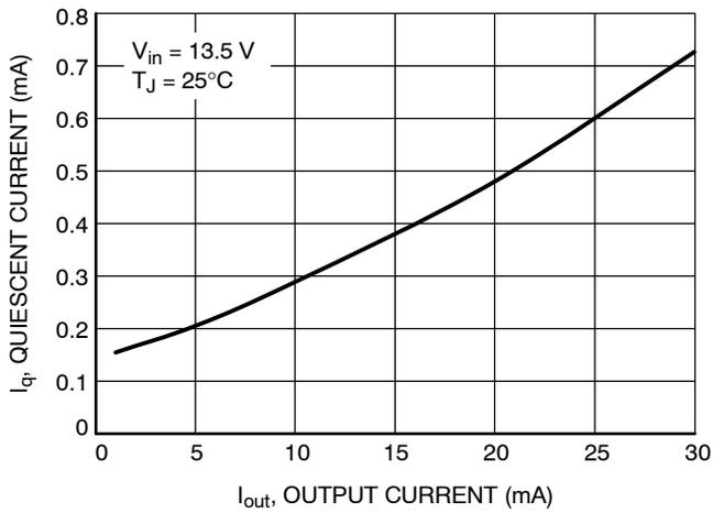
Figure 8. Quiescent Current vs. Output Current (High Load)
