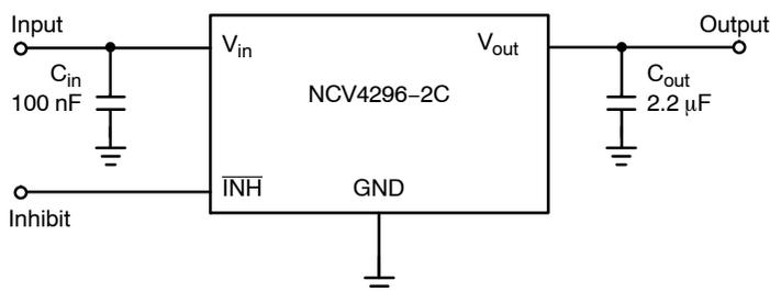
Figure 1. Applications Circuit
