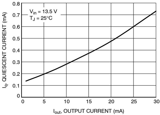
**Figure 16. Quiescent Current vs. Output Current (High Load)**
