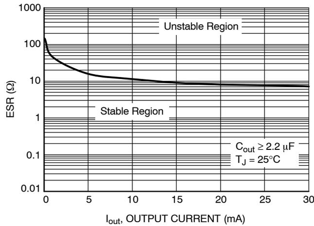
Figure 11. Output Stability with Output Capacitor ESR
