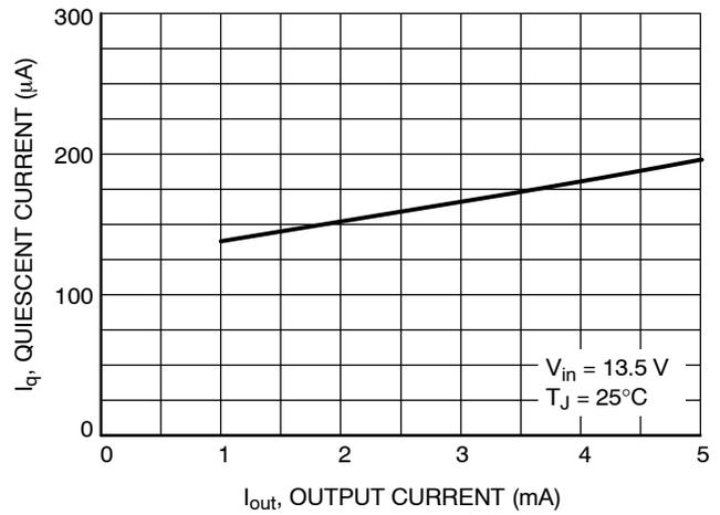
**Figure 17. Quiescent Current vs. Output Current (Low Load)**
