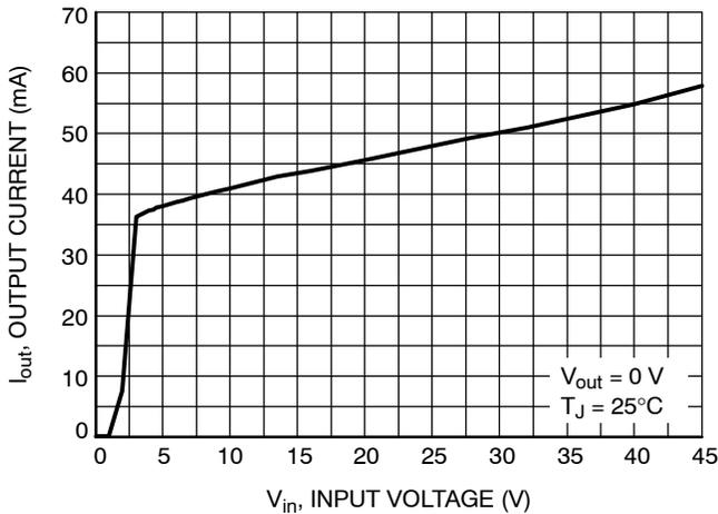
Figure 14. Maximum Output Current vs. Input Voltage
