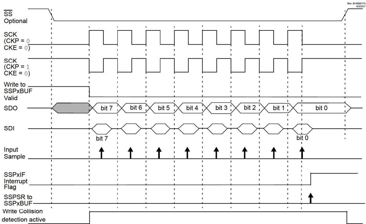
**Figure 25-8. SPI Mode Waveform (Client Mode with CKE = 1)**
