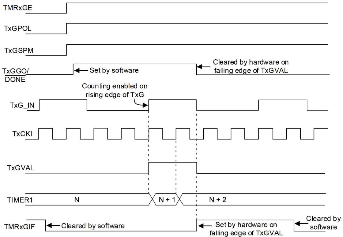
Clearing the GSPM bit will also clear the **GGO/DONE** bit. See the figure below for timing details. Enabling the Toggle mode and the Single Pulse mode simultaneously will permit both sections to work together. This allows the cycle times on the Timer1 gate source to be measured. See the figure below for timing details.
