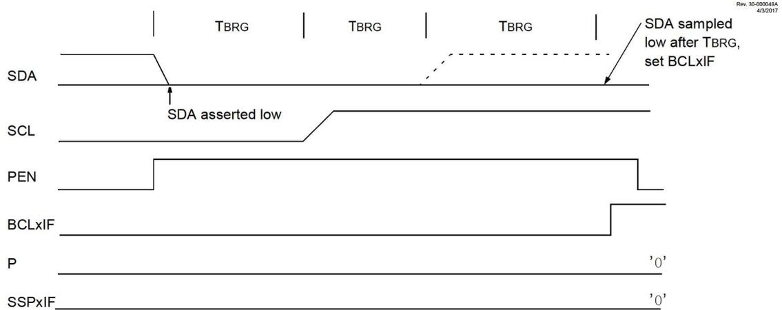
**Figure 25-41. Bus Collision During a Stop Condition (Case 2)**
