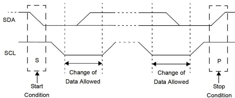
**25.2.2.9 Start/Stop Condition Interrupt Masking**
