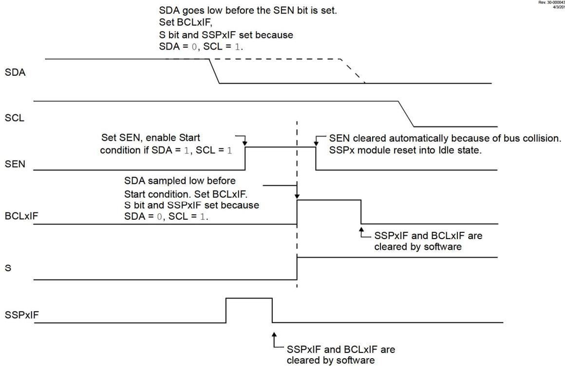
The Start condition begins with the SDA and SCL pins deasserted. When the SDA pin is sampled high, the Baud Rate Generator is loaded and counts down. If the SCL pin is sampled low while SDA is high, a bus collision occurs because it is assumed that another host is attempting to drive a data '1' during the Start condition.
