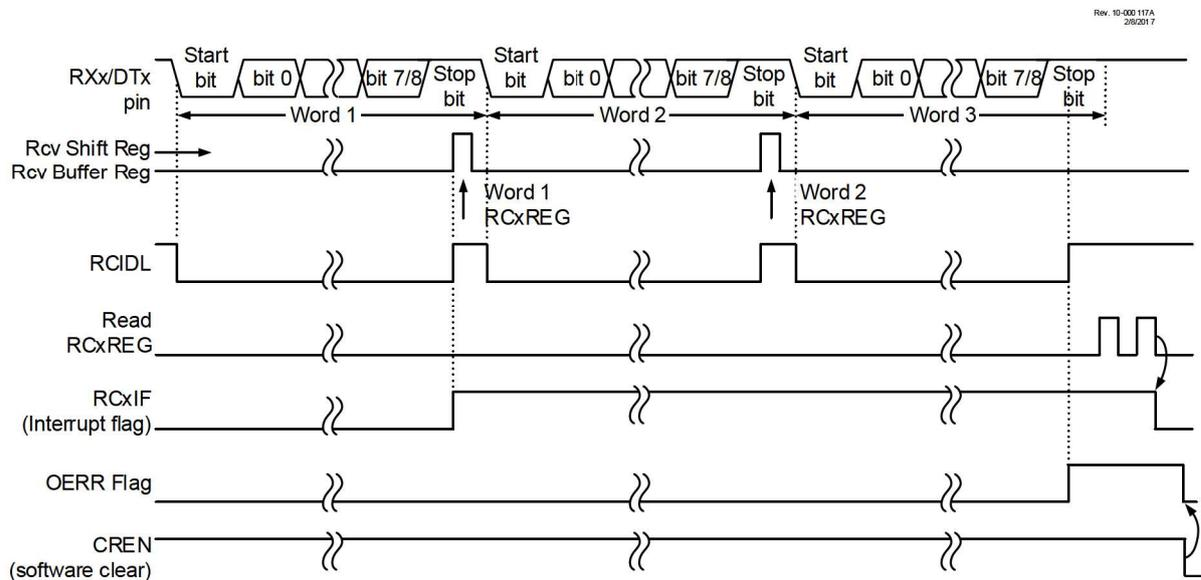
**Note:** This timing diagram shows three bytes appearing on the RXx input. The OERR flag is set because the RCxREG is not read before the third word is received.
