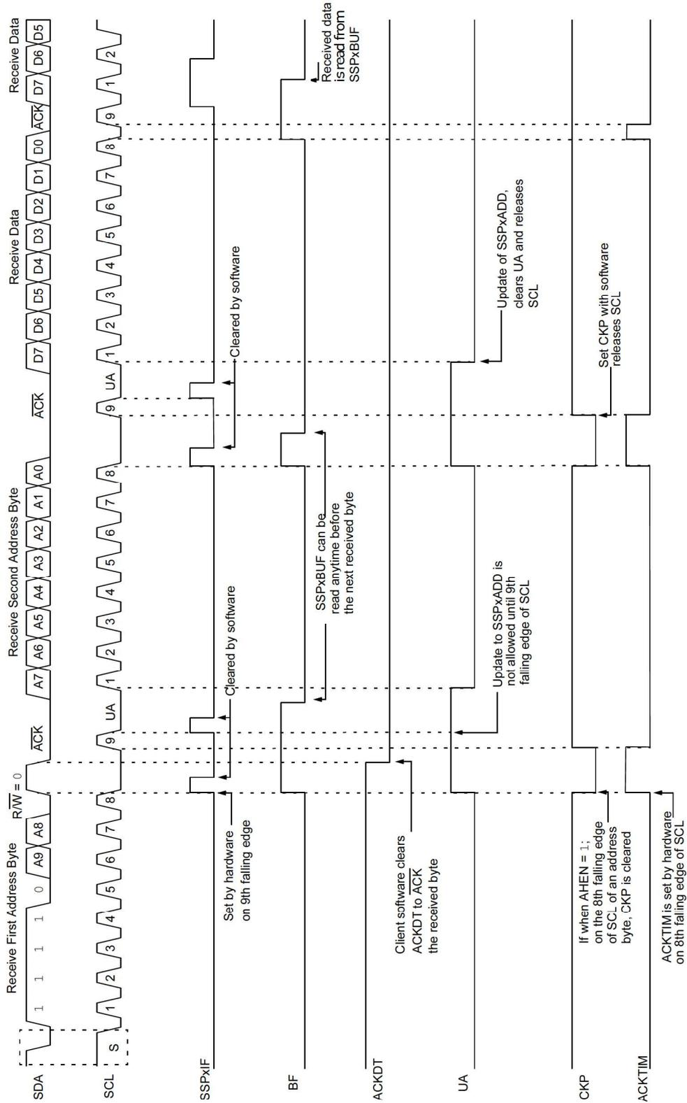
Figure 25-22. I<sup>2</sup>C Client, 10-Bit Address, Transmission (SEN = 0, AHEN = 0, DHEN = 0)
