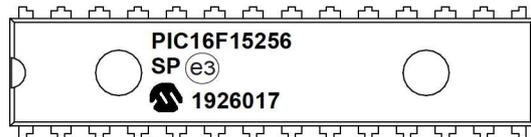
28-Lead SOIC (7.50 mm)
