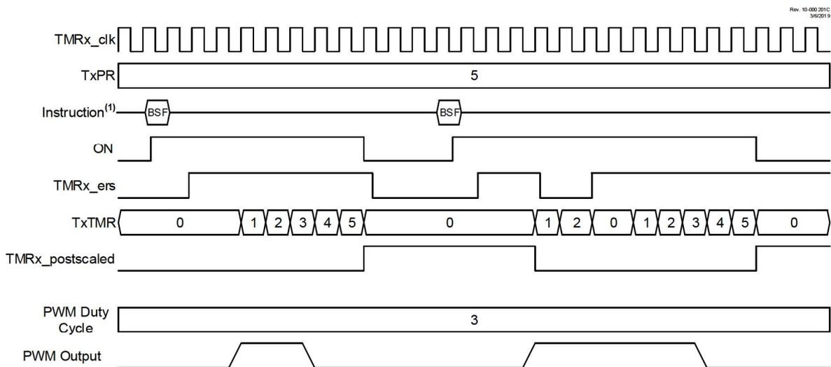
Note 1: BSF and BCF represent Bit-Set File and Bit-Clear File instructions executed by the CPU to set or clear the ON bit of TxCON. CPU execution is asynchronous to the timer clock input.
