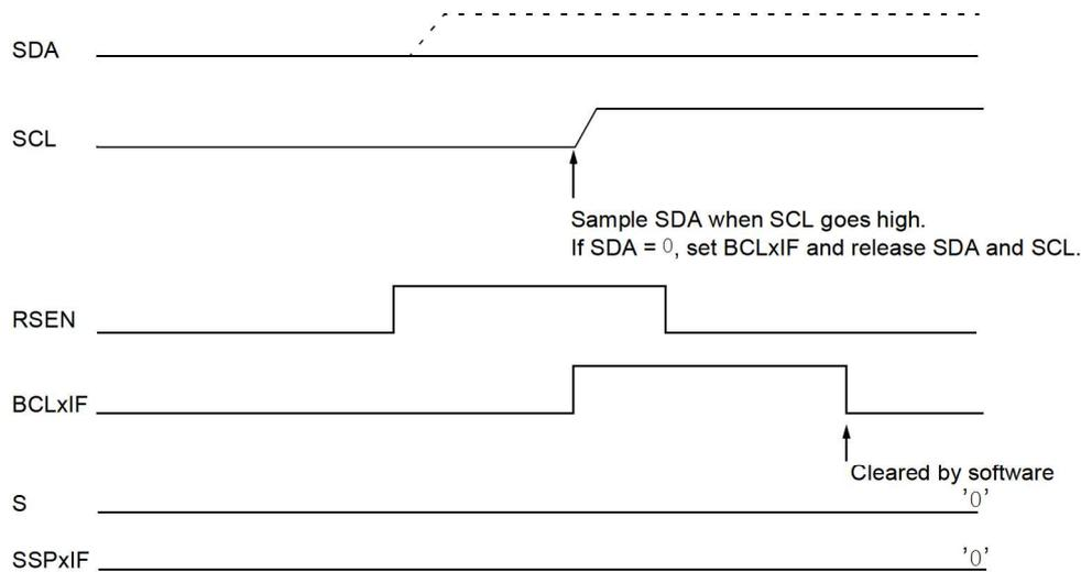
If SCL goes from high-to-low before the BRG times out and SDA has not already been asserted, a bus collision occurs. In this case, another host is attempting to transmit a data '1' during the Repeated Start condition (see [Figure 25-39](#)).
