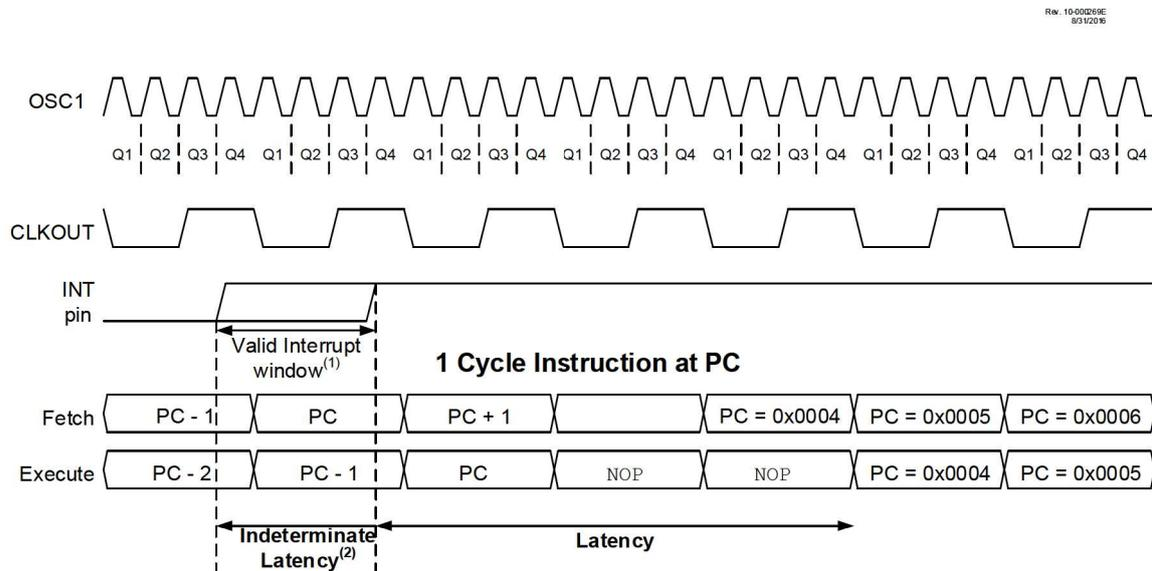
Figure 12-3. INT Pin Interrupt Timing
