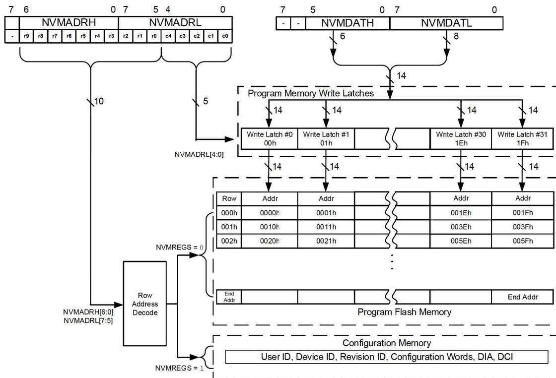
Figure 15-5. Program Flash Memory Write Sequence
