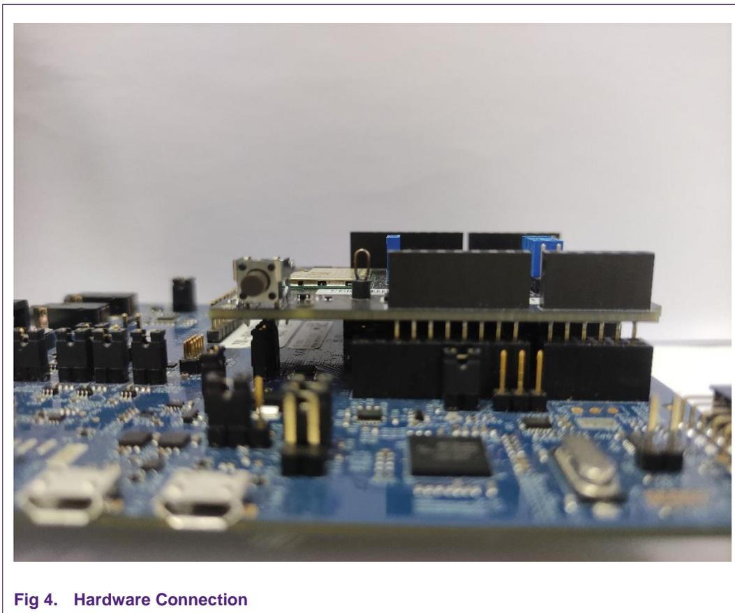
Insert the Micro-USB cable that came with the kit into the LPC55S16 EVK J1 Port (LINK2 Port), and connect it to your computer. You should see the USI Development Board's status and power LEDs light up.
