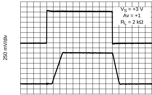
Figure 24. 3 V Non-Inverting Large Signal Pulse Response
