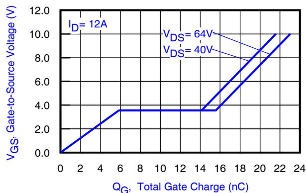
Fig 2. Total Gate Charge vs. Gate-to-Source Voltage
