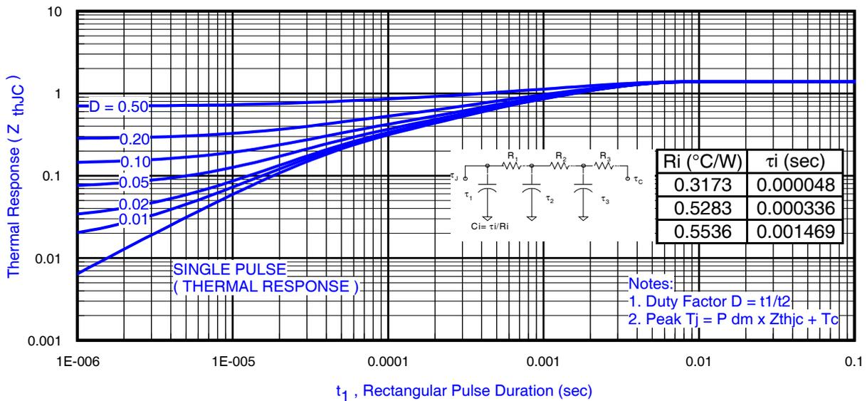
**Fig 3.** Maximum Effective Transient Thermal Impedance, Junction-to-Ambient
