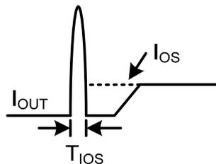
**Figure 2: Short Circuit Response Time**
