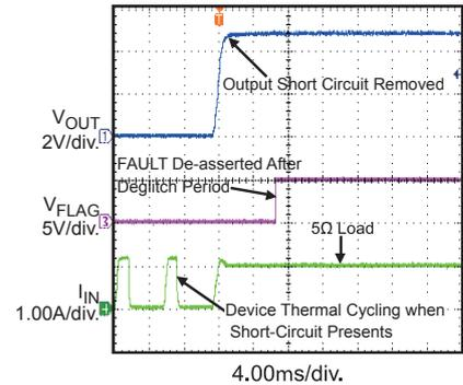
**No-Load to Short-Circuit Transient Response**
