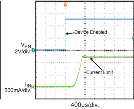
**1 $\Omega$  Load Connected to Enabled Device**
