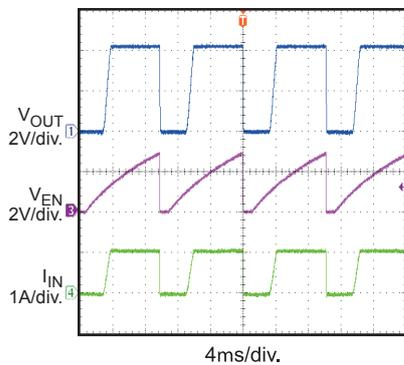
**Figure 7: Auto-Retry Waveform**
