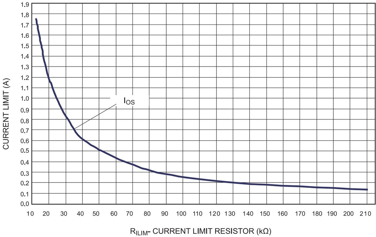
**Figure 5 : Current-Limit vs R<sub>LIM</sub>**
