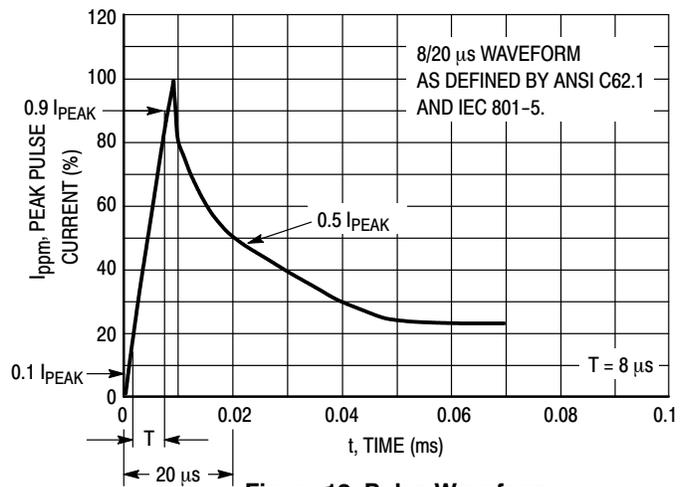
Figure 12. Pulse Waveform
