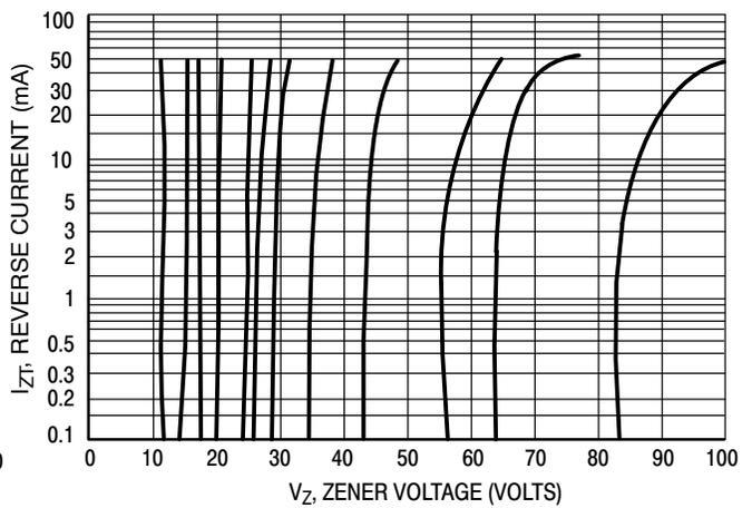
Figure 6.  $V_Z = 12$  thru 82 Volts
