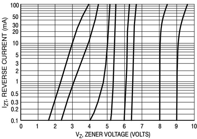
Figure 5.  $V_Z = 3.3$  thru 10 Volts
