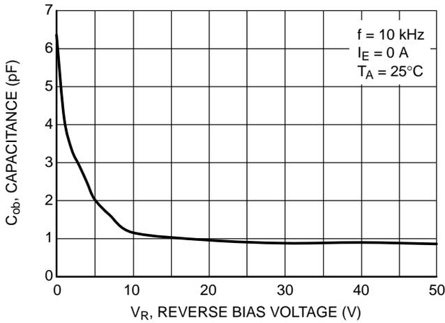
Figure 9. Output Capacitance
