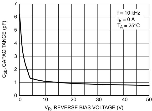
Figure 4. Output Capacitance
