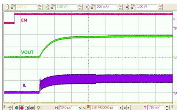
Figure 25. Startup, 3 \Omega Load
