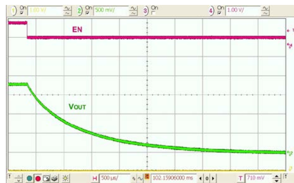
Figure 27. Shutdown, No Load, Output Discharge Enabled
