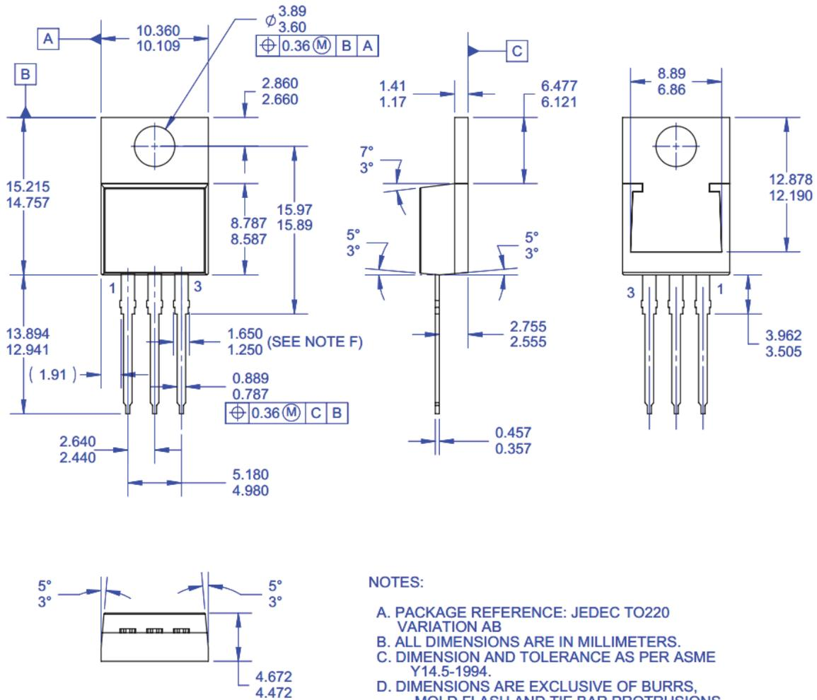
**Figure 18. TO-220, Molded, 3-Lead, Jedec Variation AB (Delta)**
