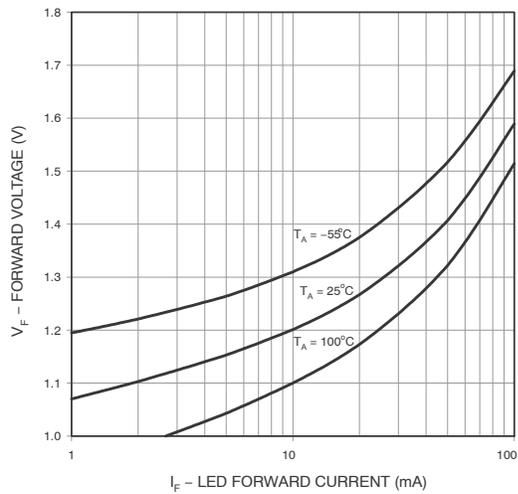
Figure 2. LED Forward Voltage vs. Forward Current
