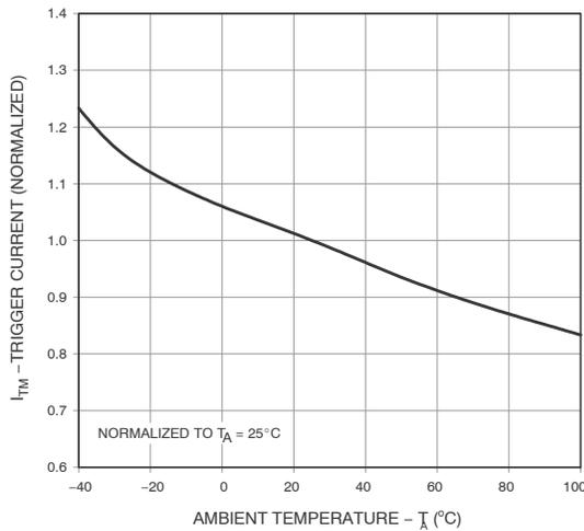
Figure 4. Trigger Current vs. Ambient Temperature
