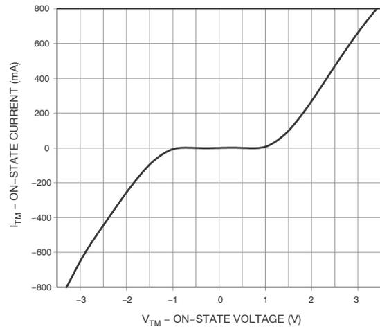
Figure 3. On-State Characteristics
