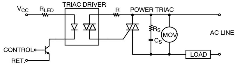
Typical Snubber values  $R_S = 33 \Omega$ ,  $C_S = 0.01 \mu F$
