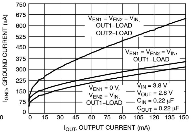
Figure 6. Ground Current vs. Output Current -
