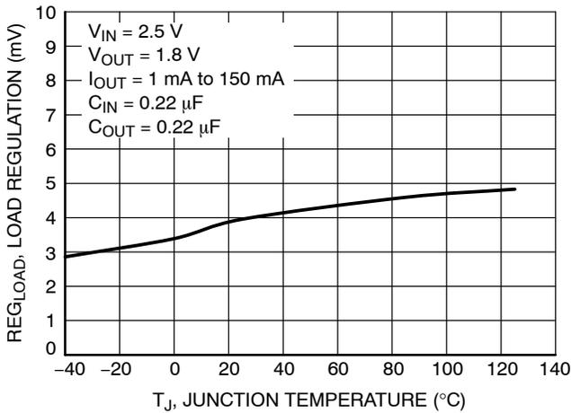
Figure 11. Load Regulation vs. Temperature
