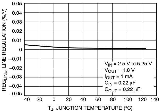
Figure 8. Line Regulation vs. Temperature
