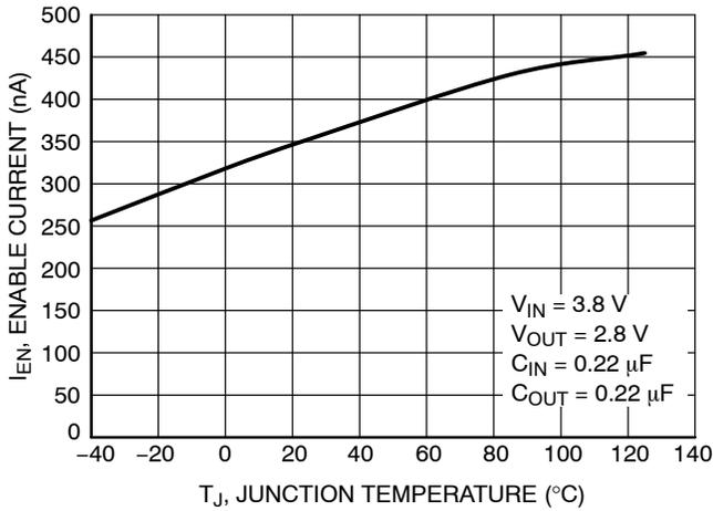
Figure 21. Current to Enable Pin vs. Temperature
