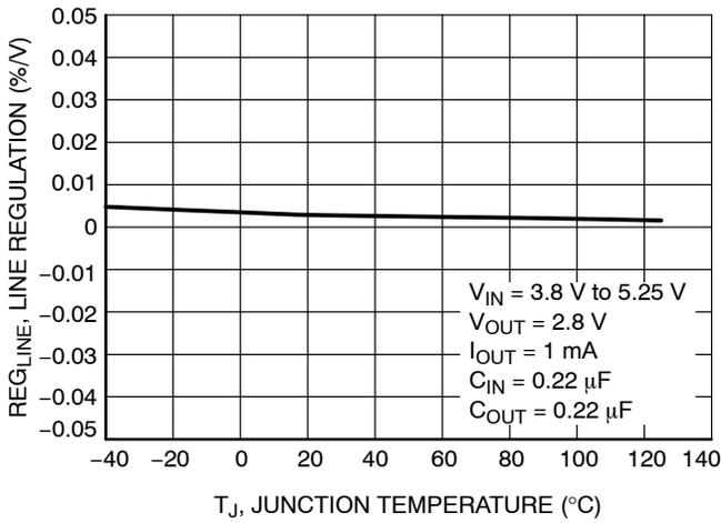
Figure 9. Line Regulation vs. Temperature
