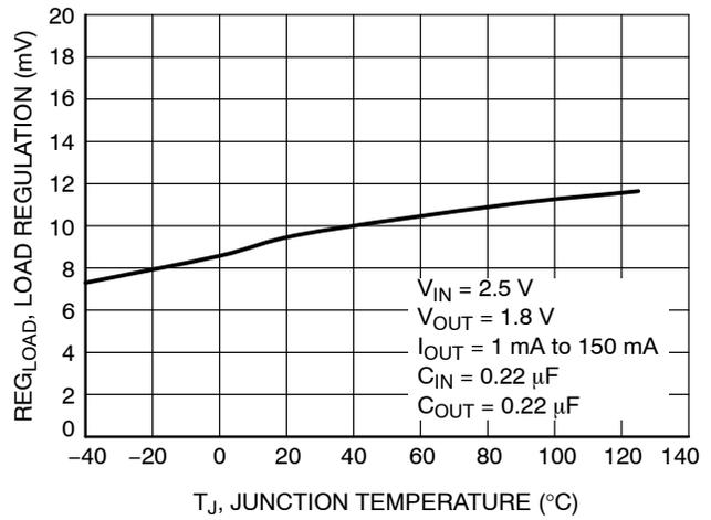
Figure 10. Load Regulation vs. Temperature
