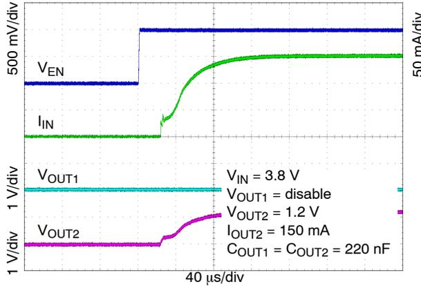
Figure 34. Enable Turn-on Response - VR1 = Off, VR2 = 150 mA
