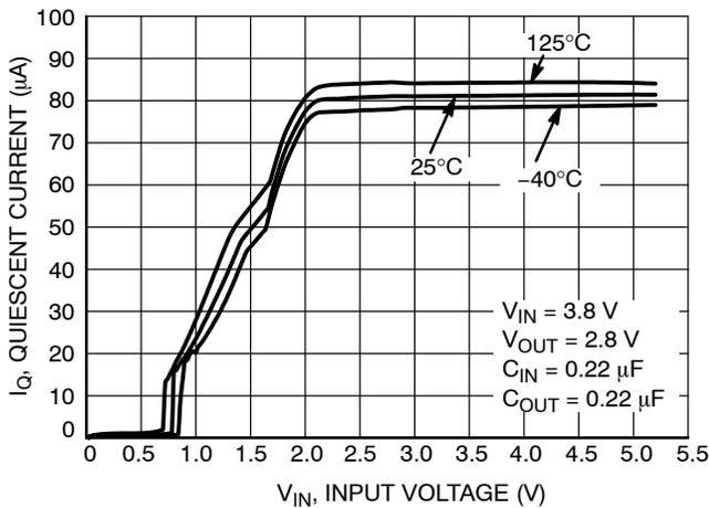
Figure 7. Quiescent Current vs. Input Voltage -
