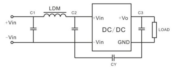
Note 2: C1,C2 are 4.7uF/50V, LDM is 6.8uH, CY is 1nF/250Vac, for C3, please refer to the Typical Circuit.
