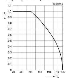
Maximum I<sub>BMS</sub> current as function of the ambient temperature: I<sub>BMS</sub> (T<sub>A</sub>) = Factor × I<sub>BMS</sub> (70 °C)
