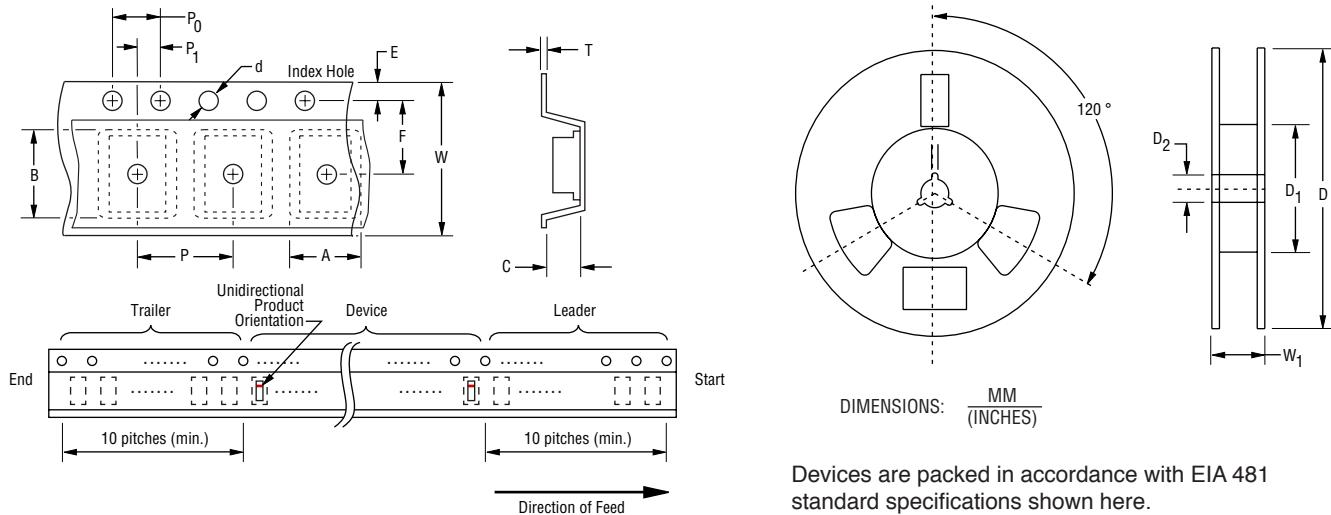
Devices are packed in accordance with EIA 481 standard specifications shown here.
