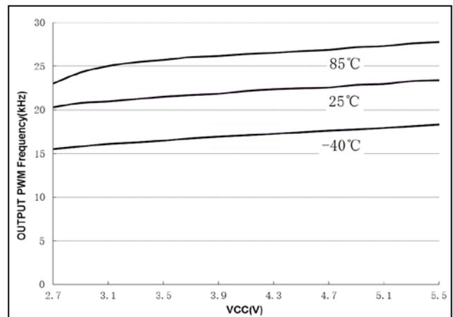
**Figure 8** V<sub>CC</sub> vs. Output PWM Frequency
