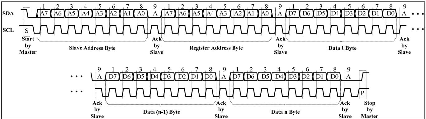
Figure 5 Writing to IS31FL3236A (Automatic Address Increment)
