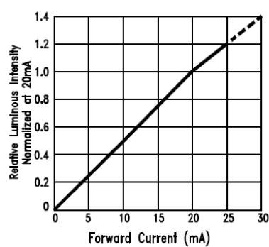
Fig.4 Relative Luminous Intensity
