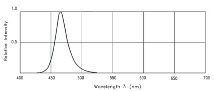
Fig.1 RELATIVE INTENSITY VS. WAVELENGTH
