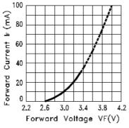
Fig.2 FORWARD CURRENT VS. FORWARD VOLTAGE
