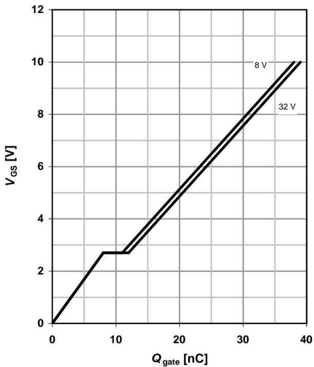
**16 Gate charge waveforms**
