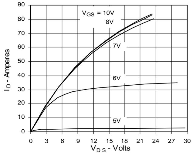
**Fig. 3. Output Characteristics**
