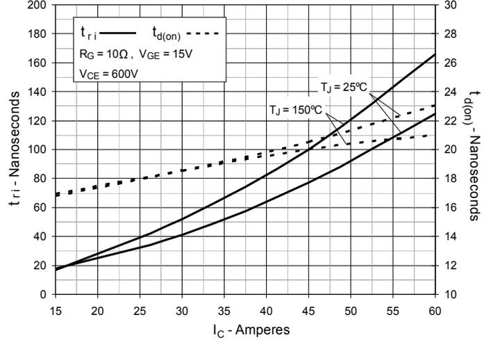
**Fig. 20. Inductive Turn-on Switching Times vs. Junction Temperature**
