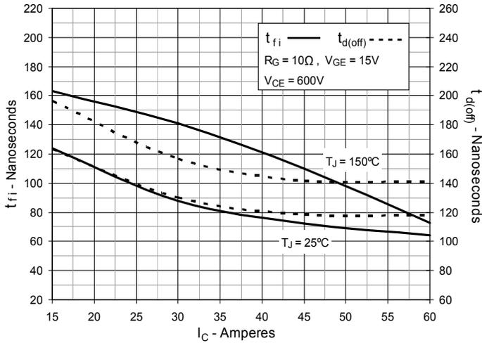
**Fig. 17. Inductive Turn-off Switching Times vs. Junction Temperature**
