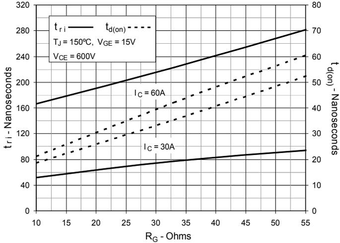
**Fig. 19. Inductive Turn-on Switching Times vs. Collector Current**
