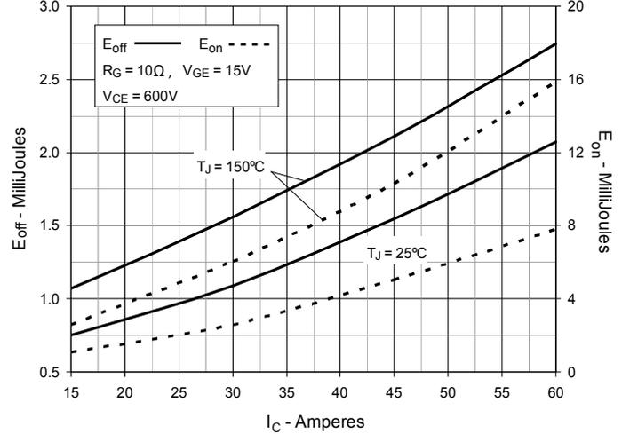
**Fig. 14. Inductive Switching Energy Loss vs. Junction Temperature**
