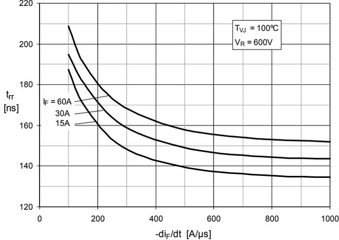
**Fig. 28. Peak Forward Voltage  $V_{FR}$ ,  $t_{rr}$  vs  $-di_F/dt$**
