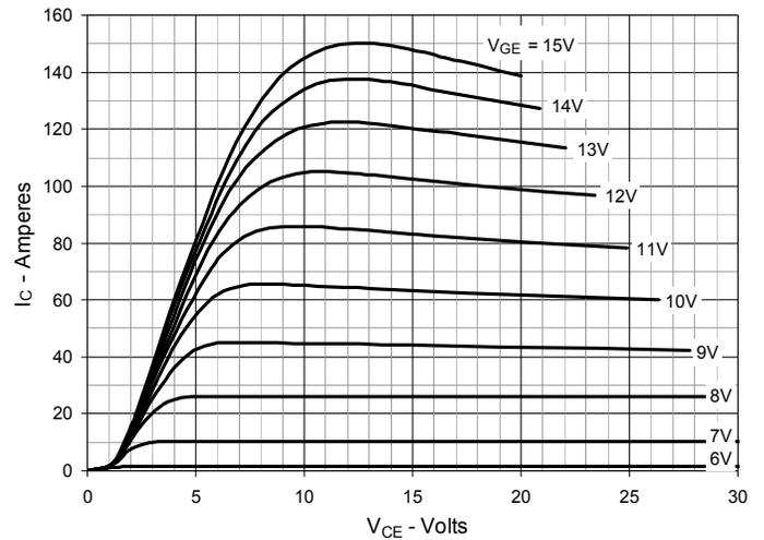
**Fig. 3. Output Characteristics @  $T_J = 150^\circ\text{C}$**
