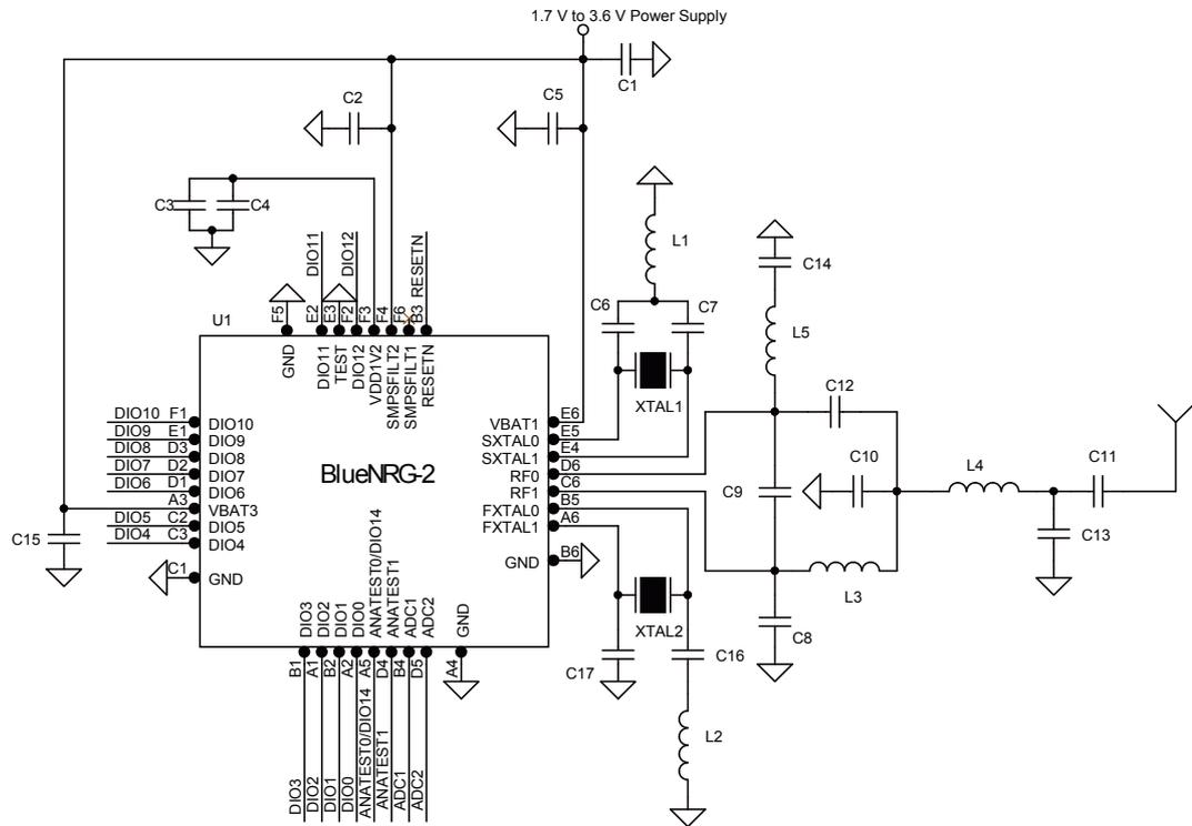
Figure 30. Application circuit: active DC-DC converter QFN32 package with BALF-NRG-02D3 balun
