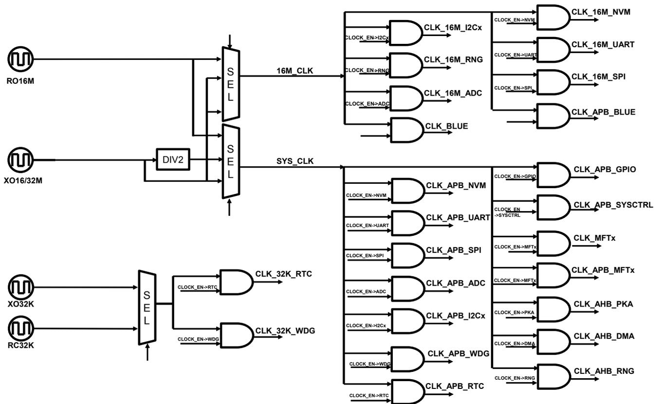
*Note:* When 32 MHz XO is used, the Cortex-M0, the DMA and the APB tree (except for BLE radio access) run at 32 MHz. The rest of the clock tree is divided by two and is at 16 MHz.
