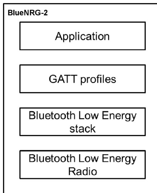
The BlueNRG-2 can be configured to operate as a network coprocessor. In this case, dedicated firmware is provided to support the interface with an external application processor. The whole Bluetooth low energy stack runs in the BlueNRG-2; the GATT profiles are provided to run in the application processor together with the application code. The figure below shows the network processor RF software layers.
