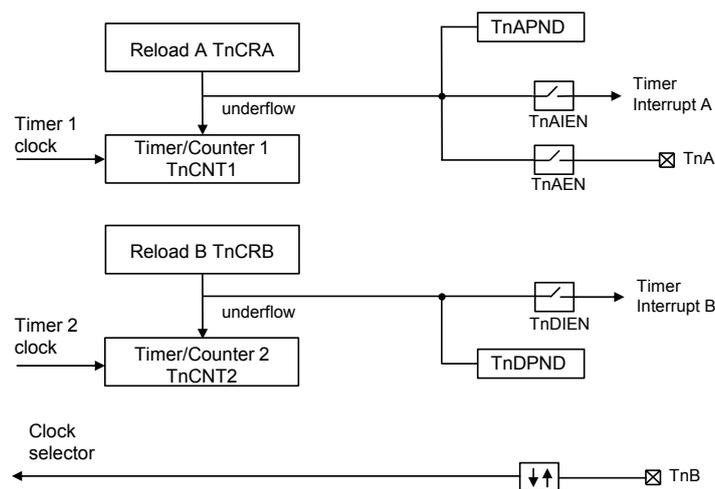
In mode 3, the Timer/Counter is configured to operate as a dual independent system timer or dual external-event counter. In addition, the Timer/Counter 1 can generate a 50% duty cycle PWM signal on the TnA pin. The TnB pin can be used as an external-event input or pulse-accumulate input, and serve as the clock source to either Timer/Counter 1 or Timer/Counter 2. Both counters can also be operated from the prescaled system clock.
