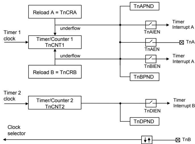
In this mode, the timer toggles the TnA output upon underflow, which is connected to PWMx pin of the device. This generates a clock signal on TnA with the width and duty cycle controlled by the values stored in the TnCRA and TnCRB registers.
