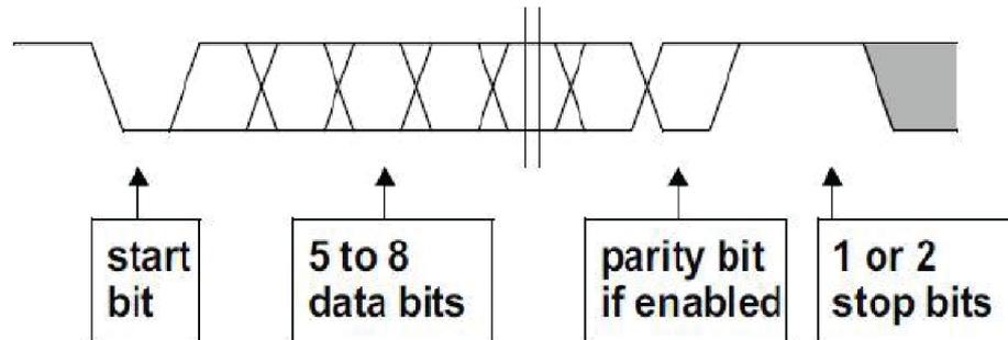
The FIFOs can be disabled. In this case, the transmit and receive sides of the UART have 1-byte holding registers (the bottom entry of the FIFOs). The overrun bit is set when a word has been received, and the previous one was not yet read. In this implementation, the FIFOs are not physically disabled, but the flags are manipulated to give the illusion of a 1-byte register.
