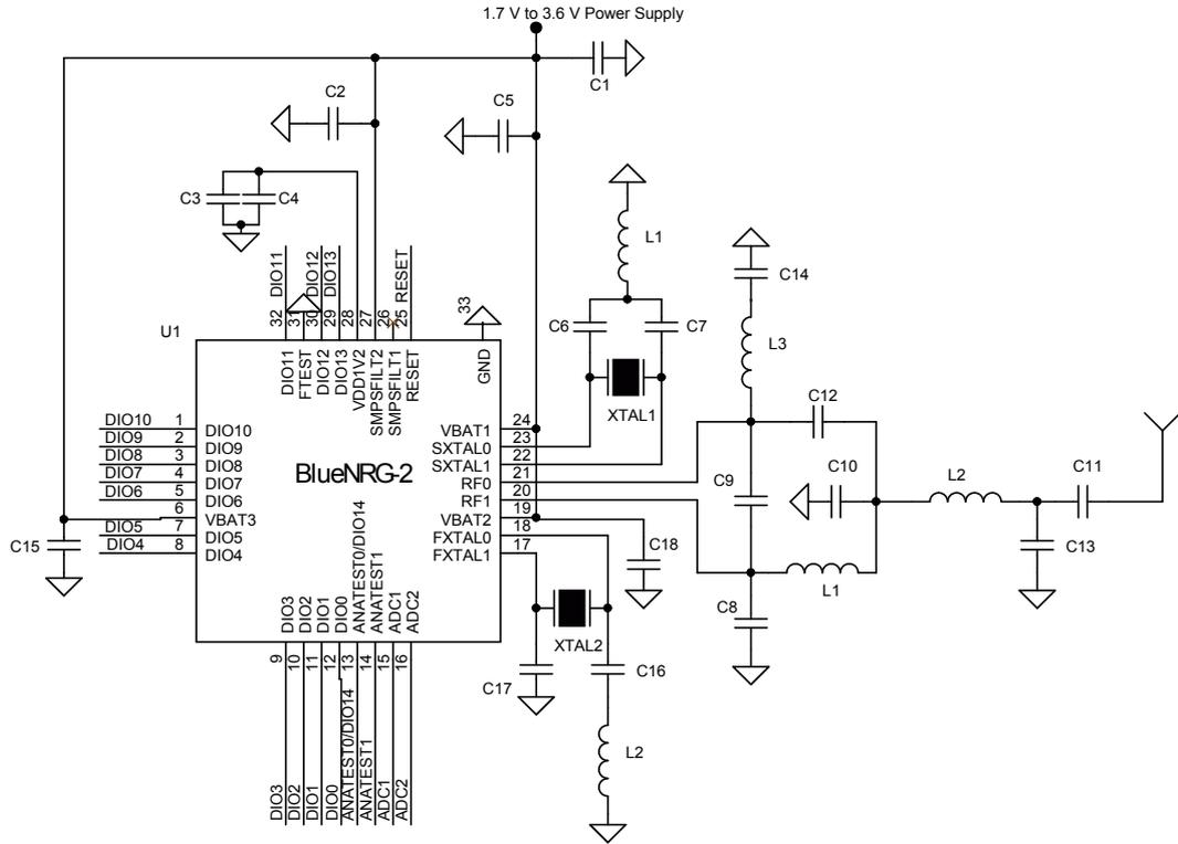
Figure 28. Application circuit: active DC-DC converter WCSP34 package
