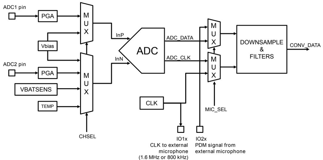
Several channels are available for the conversion, the CHSEL selects the channel according to [Table 25. ADC channels](#).
