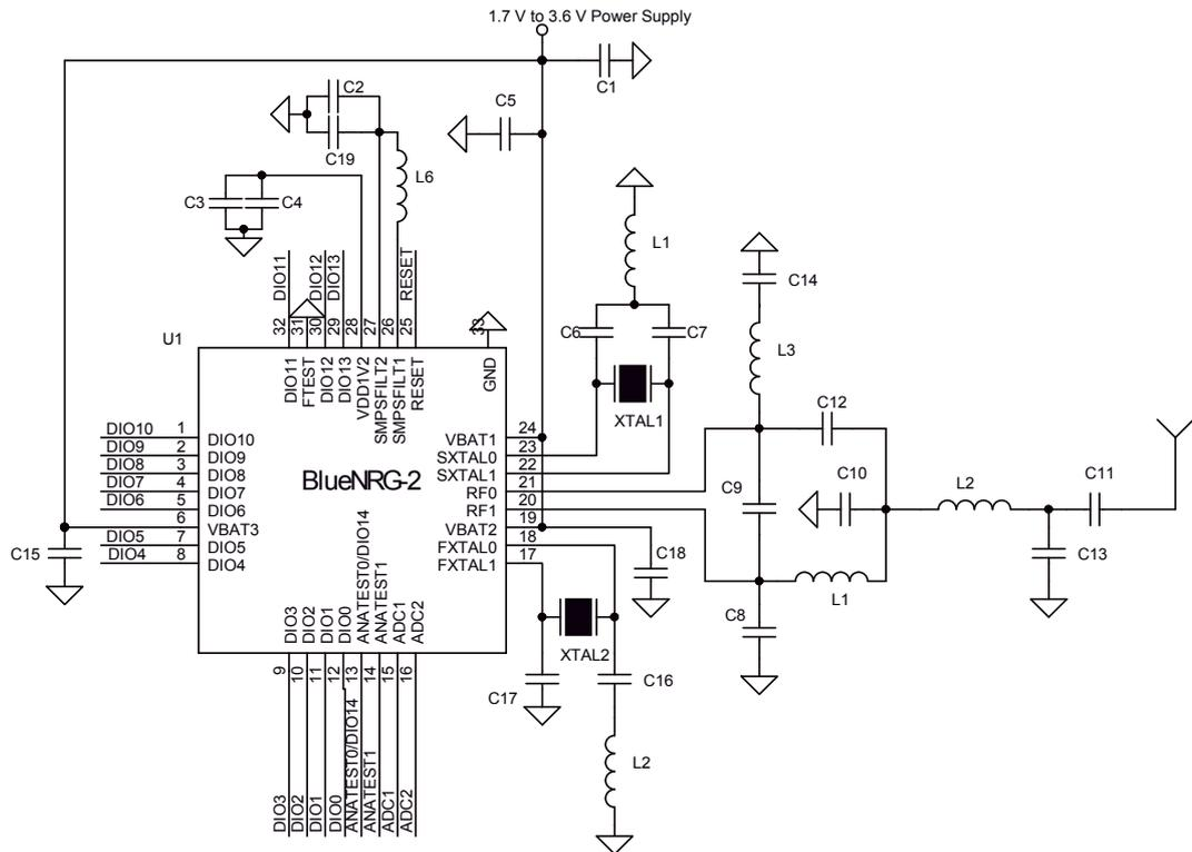
Figure 27. Application circuit: non-active DC-DC converter QFN32 package
