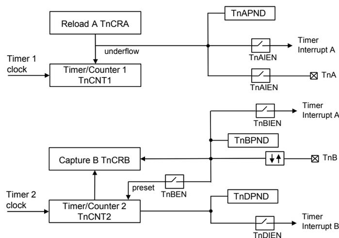
This mode is a combination of mode 3 and mode 2, and makes it possible to operate Timer/Counter 2 as a single input-capture timer while the Timer/Counter 1 can be used as a system timer as described above.
