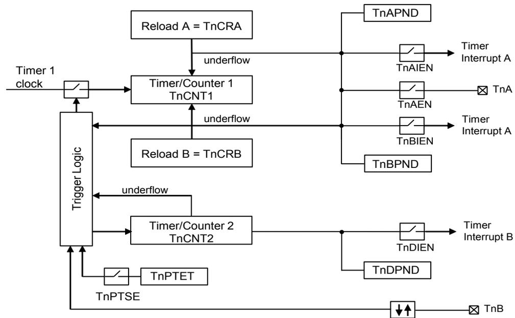
In mode 1a, Timer/Counter 2 behaves differently from the way it behaves in the other modes. If an underflow condition occurs, the counter is preset to 0x0000 and not 0xFFFF.
