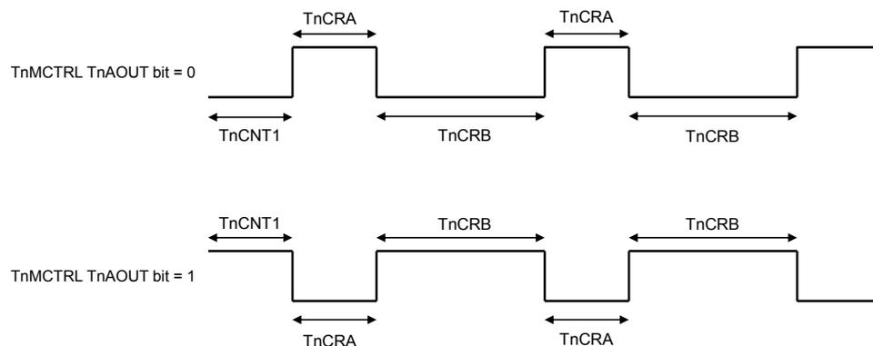
When started, the first time the Timer/Counter 1 starts with preprogrammed value in the register TnCNT1 and count down at the clock rate selected by the Timer/Counter 1 clock selector (TnCKC register). When an underflow occurs, the TnCNT1 register is reloaded alternatively with TnCRA and TnCRB registers (in this order) and counting proceeds downward from the loaded value.
