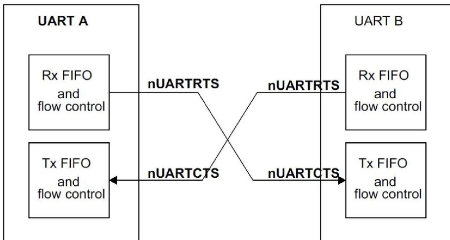
When the RTS flow control is enabled, the UART\_RTS signal is asserted until the receive FIFO is filled up to the programmed watermark level. When the CTS flow control is enabled, the transmitter can only transmit data when the UART\_CTS signal is asserted.
